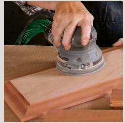
**Flat surfaces first.** It is fine to use a power sander on the raised portion of the panel and its back.
