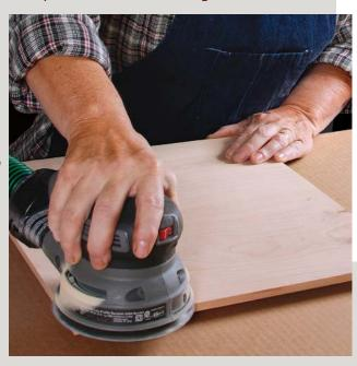
Check the surface. Looking across the surface into a raking light (above) helps reveal any imperfections. This pigtail squiggle (right) was probably caused by a piece of debris that the sander picked up when it was set down on the bench. long enough, it becomes 120 or 150 grit. It just creates 100-grit scratches, more and more slowly.
