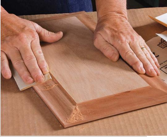
**Hand-sand the profile.** Don't use the sander, even on a flat, bevel-edged profile. Instead, hand-sand up to the same final grit as used on the sander. Go to 320 or 400 grit on the end-grain sections, so they don't absorb too much finish and end up darker than their surroundings.
