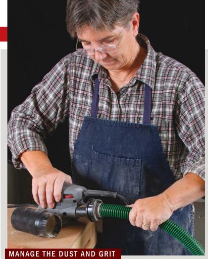
**Attach a vacuum.** As well as keeping your lungs cleaner, attaching a vacuum lets sanders cut faster and extends the disk's lifespan.
