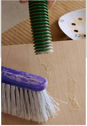
Clean between grits. Remove any dust left on the workpiece before switching to a higher grit. It reduces the risk of coarse abrasive contaminating the finer disk, and it keeps the shop cleaner.
