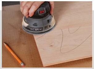
**Then smooth.** After you've removed surface imperfections with a coarse grit, the role of subsequent finer grits is to refine the scratch pattern. Here's a great way to know when to switch grits. Draw a light pencil line across the surface and sand the whole surface until the line is gone. Repeat and then move on to the next-grit disk.
