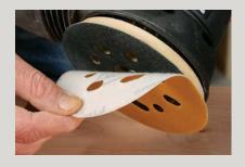
Years ago, pressure-sensitive adhesive (PSA) disks were cheaper than hook-and-loop (H&L) ones, but if you were sanding a small piece you often had to discard a PSA disk before it was used up, whereas H&L disks can be reused. Now the cost has nearly evened out and most sanders
