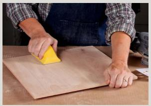
**Hand-sand last.** Once you've completed the final grit with the sander, use a sanding block with the same size grit, sanding with the grain. This removes any swirls left by the sander. Finally, use 180- or 220-grit paper and a sanding block to break the edges. Don't attempt this with a sander.
