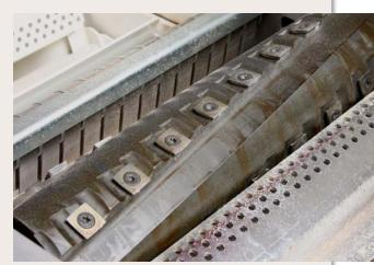
Next-generation cutterheads are available. Segmented cutterheads are starting to appear in lessexpensive jointer-planers, such as the Grizzly G0634XP. The carbide teeth last much longer than steel knives, and are easily rotated to a fresh edge.
