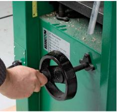
Changeover is easy. You just slide the fence to the rearmost position and the cutterhead guard to the front. Then you lift only the jointer outfeed table into position (left). As with all the machines, you must move the planer bed to reposition the dust collection, but the Rikon's aggressive screw pitch speeds the process (right).
