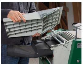
Got an empty shelf? The jointer outfeed table, along with the fence, must be removed and stored to change from jointing to planing mode.
