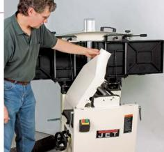
**Flip.** A single dust chute rotates around the cutterhead to handle jointing or planing, a convenient design.
