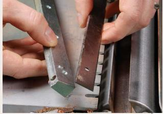
Most use straight knives. It can be tricky to re-install and adjust the knives after they've been sharpened. Disposable knives, like those on the Rikon 25-010, are a bit easier to set up, but they must be replaced when dull.
