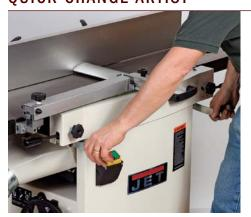
**Unlock.** Two levers keep the jointer beds fixed in place. Release them to switch from jointing to planing mode.
