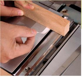
**Set the depth of cut.** Lower the outfeed table until a block of wood (representing the sharpening stone) just touches the knife. A strip of copier paper should just slip under the wood at the start of the outfeed table.
