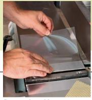
Protect the table. Apply some self-adhesive, plastic laminate sheet (leevalley.com) to the start of the outfeed table. This will protect it from the sharpening stones. If you are just lightly honing the knives, clear packing tape works fine.
