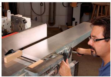
**Move the table.** This will rotate the knife forward, so it ends up about ½ in. below a block of wood representing the sharpening stone. Now you can hone the bevel at an angle that won't rub on the workpiece.
