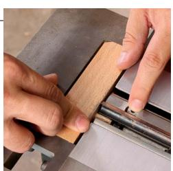
**Insert locking jig.** With the machine unplugged, the infeed table all the way up, and one of the knives at its apex of its arc, test-fit the jig.
