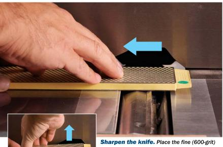
**Sharpen the knife.** Place the fine (600-grit) side of the diamond stone on the knife with about half its length on the outfeed table. You can also use water- or oilstones, or sandpaper on plywood. Draw the stone toward the outfeed table, to avoid creating a burr (below, left). Lift the stone back over the knife and repeat the step.
