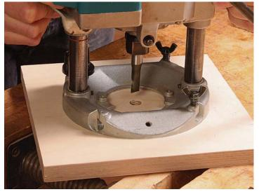
**First, plunge through a square base.** Put a ½-in., plunge-cutting bit in the collet, and plunge down through the base.
