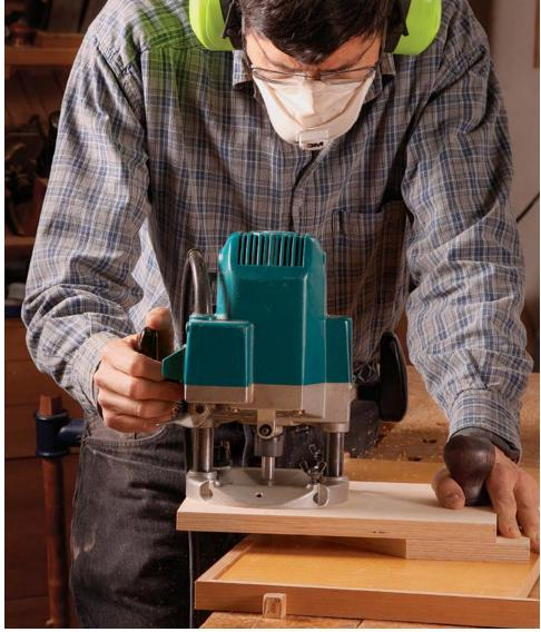
**Trim solid edging.** The angled front on the bottom layer lets Miller work all the way into the corners on this veneered top. He starts with a climb cut on the outermost edge to reduce tearout. The bit is set to leave just a bit of edging to be scraped and sanded flush.
