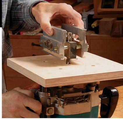
**An unlikely layout tool.** With a ½-in. drill bit chucked in the router, Miller uses a doweling jig to locate and drill the pin holes directly opposite one another and equidistant from the bit.
