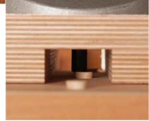
**Sure-footed.** The base straddles a series of screw-hole plugs, for example, with the twin support rails preventing the bit from tipping into the work surface.
