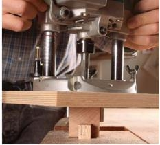
Rotate the router. When the pins touch the sides of the workpiece, the router bit is centered.
