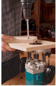
**Elevate the base.** Adding a partial bottom layer (above) prevents the base from bumping into the projections you want to trim flush, like the solid edging on the veneered panel at right.
