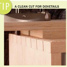
A bottom layer with a straight front edge is great for flush-trimming dovetails.
