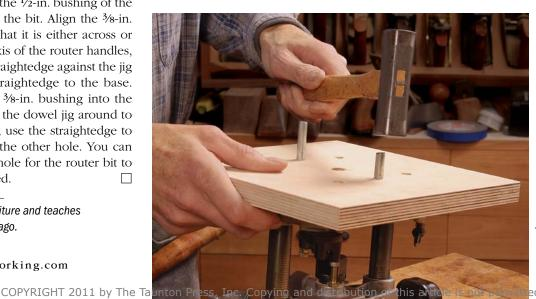
Pins center the router. Add some glue, drive in two 3%-in. dowels or metal pins, and the jig is done.
