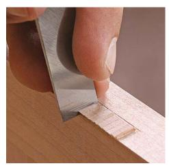
**Chop across the grain.** It's easier to control the cut depth this way.
