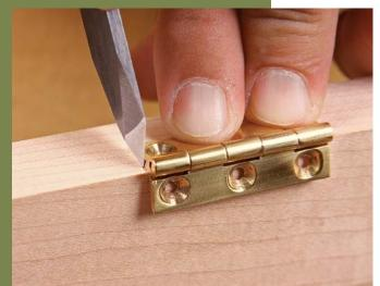
They cut the wrong wood. For accuracy, the flat back of the knife must go against the hinge. That means the bevel faces out, slicing wood fibers that aren't part of the mortise.
