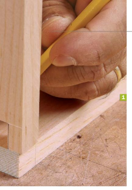
is wood that I want to keep. If you trace the pins with a knife, pressing it firmly against the pins, you cut into wood that will be part of the tails. If you later remove that scribe line when paring the tails, the joint may be too loose. If you leave it, then there will be a small gap visible, created by the beveled edge of the knife. (The same is true for a hinge mortise. As you scribe around the leaf, the knife cuts into a part of the stile that needs to be kept.)
