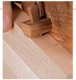
**But it's OK to scribe for the side.** The bevel on a marking gauge's cutter faces the waste wood, so paring away the entire cut line creates a mortise of the perfect width.
