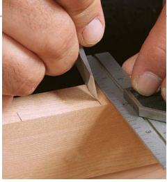
**Add a knife line for easier paring.** Put the knife on the inside of the line (above), push the square against it, and then scribe the line (right).
