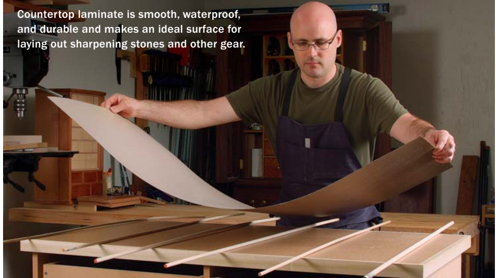
Laminate is an excellent choice. Use dowels to line up the laminate before affixing it in place with contact cement.
