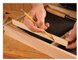
**Finishing touches.** A layer of rubber mesh drawer liner cushions the tools and helps keep them from sliding. After marking and cutting the pieces to length (above), profile the dividers as needed for easy access to the tools and slide them into place (right).
