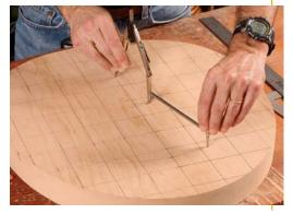
chair, the circle has a diameter of 12 in. and is located  $1\frac{1}{2}$  in. from the center of the mortise for the seat post.
