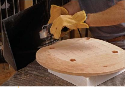
Grind a curve onto the edge. Kamerath raises the seat blank on a block of foam so the grinder doesn't dig into his bench (above). Check for symmetry after redrawing the grid, marking the high spots with a pencil (right).
