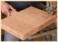
Rough out the shape. From here, the shaping process is identical to how you made the seat.
