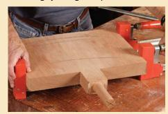
Glue the three parts together. After turning a tenon on the narrow center post, glue a "wing" to both sides.
