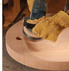
Start with the grinder. It makes a big mess, but most of it can be caught by a large dust hood hooked up to a dust collector. Then sand the hollow with a P60-grit pad on a random-orbit sander (above) to remove the marks left by the grinder.
