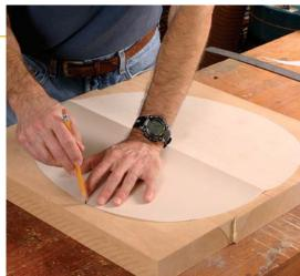
**Draw the outline first.** Use a template to guarantee symmetry. Kamerath makes his by folding a piece of vellum (available at artsupply stores) in half and cutting the shape. The fold aligns with a centerline drawn on the blank.
