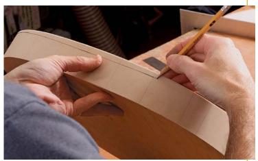
Lay out a relief on the front edge. Draw it on a piece of vellum glued to the blank temporarily with spray adhesive. Then use an aggressive grinding disk (Kamerath uses the Holey Galahad coarse disk from King Arthur's Tools; katools.com) to grind to the line. After grinding the relief, fold the vellum over on itself to check for symmetry.
