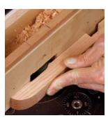
A shallow relief creates the feet. Using a stop block against the routertable fence, Becksvoort pivots into the cut and pivots out at the halfway mark. Then he flips the piece and pivots in again from the other side. This ensures that all the feet are exactly the same size.
