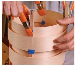
Add the top. When all the rings are dry, glue the top into its bridle joints. Spring clamps are perfect for this glue-up.
