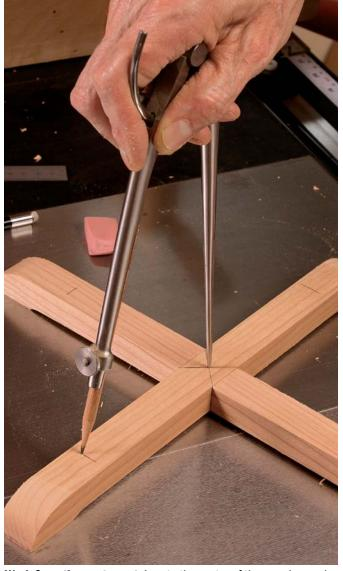
**Work from the center out.** Locate the center of the crosslap, and then use a compass to mark an equal distance on all four feet. The distance is not as important as that they all be identical.
