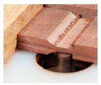
**Precise tenon.** Take several passes to sneak up on final thickness, using dial calipers to check against the mortise as you go.
