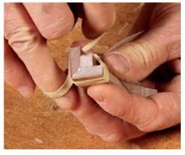
Glue up the leg. Use a glue block to reinforce the miter joint and support the box from below. Packing tape and rubber bands add clamping pressure.
