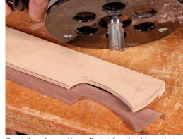
**Rout the shape.** Use a flush-trimming bit so that the leg is an exact copy of the template. After routing the first half, flip the blank end for end and rout the second one.
