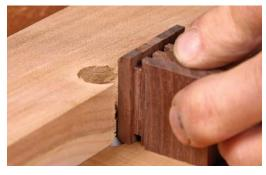
For the end grain, chamfer several pulls at once.
