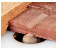
**Smooth curve.** A push block behind the blank prevents tearout and keeps it square to the fence, guaranteeing a straight cut.
