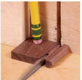
Finally, free the pull. Put a stop block on your tablesaw sled, and use a pencil to hold down the part. Push the sled until both pieces are clear of the blade and turn off the saw before moving the pull. If you pull the sled back, the blade can throw the pull.
