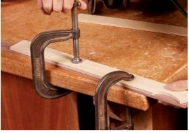
**Clamp on the template.** Place the workpiece against the fence of the template and clamp both so that they overhang the workbench.
