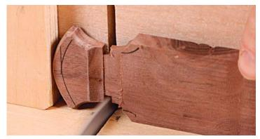
The tenon gets shoulders on all four sides. Use a stop block so that the shoulders cut at the tablesaw line up with those cut at the router table. Last, cut the pull free from the blank.
