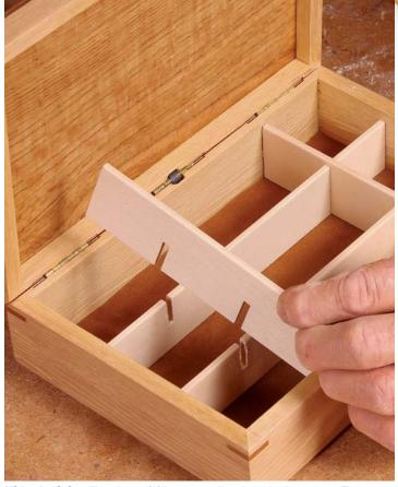
**Hide the joint.** The short dividers are taller than the long ones. That extra bit of material hides the slots.
