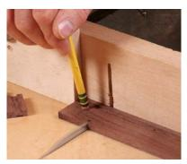
Then cut shorter blanks for the pull. Switch over to the tablesaw, using a pencil eraser to hold the cutoff piece on your crosscut sled.
