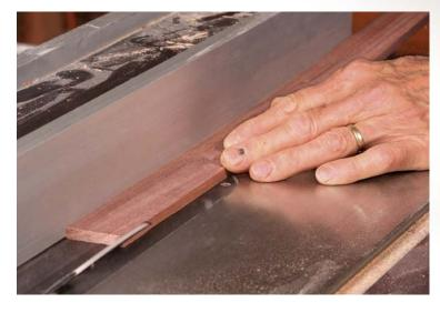
Cut the miter first. Miter the edge of a blank long enough for all eight halves needed to make the four legs.
