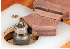
**Soften the edges.** Be sure the bearing is against the end grain when starting the cut, so the bit doesn't grab the corner.
