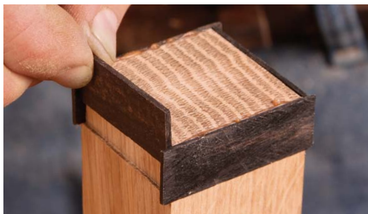
Glue the cuff stock in place. Rodel clamps two opposite sides at a time, leaving the first pair long and cutting the second pair to fit between those. Once the glue is dry, he trims the ends and sands the cuffs flush to the legs.
