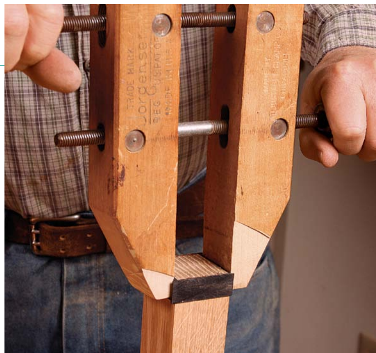
Glue the cuff stock in place. Rodel clamps two opposite sides at a time, leaving the first pair long and cutting the second pair to fit between those. Once the glue is dry, he trims the ends and sands the cuffs flush to the legs.
