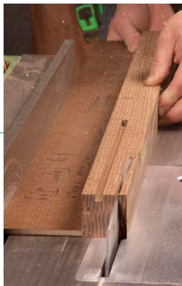
Backward taper is next. Rodel uses a simple L-shaped jig to cut the taper on the leg. Make sure your saw has its splitter in place (left).
