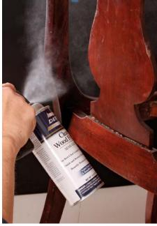
**Fine-tune the tone, and add a topcoat.** Use an aerosol toner to blend the color of the repair into the rest of the piece (left). Spray on a clear topcoat to complete the repair (right). Aerosol clear finishes come in different sheens. Apply the color and the clear coat in light bursts while holding the can farther from the surface to blend in the repair.
