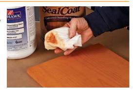
Perfectly protected. You can spray a sealer coat of shellac over even an alcohol-soluble dye and not cause any blotching.
