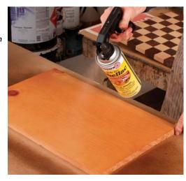
a lazy Susan. These fast-drying finishes aren't a magnet for dust and debris, and you can apply two or three coats in a day. Just don't try to apply one fat coat, or all you'll get are drips and runs.
