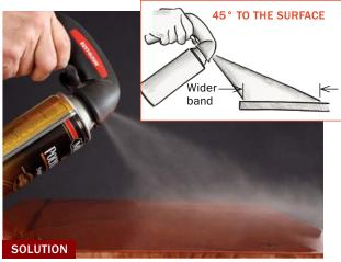
Holding the can at around  $45^{\circ}$  to the surface creates a wider spray fan on the workpiece. This helps overlap strokes to achieve an even coating, but you need to move the aerosol more slowly.
