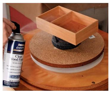
A durable topcoat. For lightly handled objects, three or four coats of solvent lacquer give plenty of protection and the finish can be done in a day. Spray the inside of the box first and the outside last. In this way, any overspray is on the less-visible surfaces.
