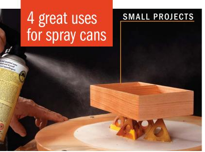
**Seal with shellac.** It is a good idea to seal bare wood with a coat of dewaxed shellac. To avoid having to touch the piece or walk around it, place it on painter's pyramids that rest on a lazy Susan.
