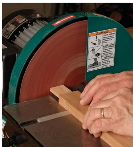
Quick trim. A disk sander trims tenons quickly. Use the miter gauge to keep the workpiece square to the disk.
