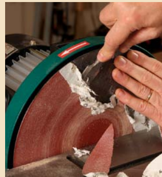
The PSA-backed sanding disks often require a fair amount of scraping to get the paper off, and leave a bit of residue behind. You can remove any adhesive residue with a solvent, such as naphtha.
