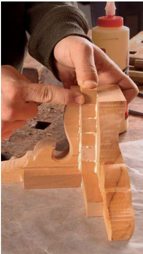
Reinforce the corners. To strengthen the miters, add glue blocks to the back of the feet. No need for clamps here; a rub joint works fine. Rub each block until the glue grabs and holds it.
