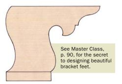
**Reference lines.** Use a full-size pattern to lay out the face profile on each end of the blank. You'll reference those lines as you rough out and refine the profile.
