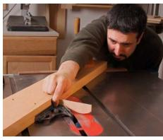
**Eyeball it.** Raise the blade to the apex of the cove. Then pivot the fence to set the cove's width, using the head of a combination square to keep the pattern 90° to the fence and table (above). Once you're there, clamp down the fence (right).
