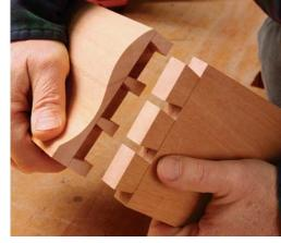
Dovetails in back. Because the rear of the case was not seen, period makers didn't bother to shape the back pieces. Those flat parts join to the shaped side pieces with dovetails.
