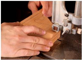
Cut the inside profile. First trim the feet to length. Then trace the pattern onto the back of each foot (above), aligning the inside edge of the pattern with the squarecut end. Cut the profile at the bandsaw (left). Work carefully—clean cuts here mean less work later.
