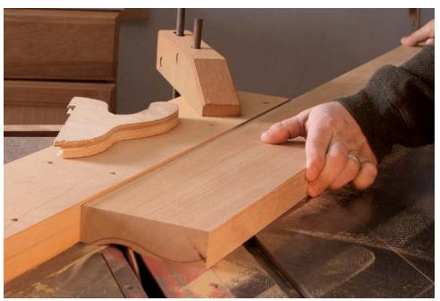
**Nibble away.** Start with the blade about ½ in. above the table. Then make multiple passes over the blade, raising it in ½-in. increments, until you've removed as much waste as possible.
