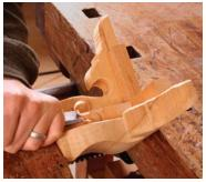
**Chamfer when dry.** A wide chamfer helps hide the glue blocks.
