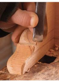
**Cleanup work.** First remove sawmarks using rasps and files (left). Use gouges to back-cut the edges slightly (center), then go back and refine only the outside profile using rasps and files. Finally, chamfer the inside edges with a chisel (right). It's OK to leave unseen, inside surfaces rough.
