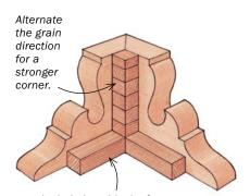
Include long blocks for gluing or screwing the feet to the case.
