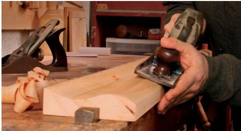
plywood, which will guide both machine and handwork (to learn more about designing ogee bracket feet, see Master Class, p. 90). I use one pattern to draw the ogee profile on each end of the blank. After the ogee shaping is complete, I use another pattern to lay out the miters and to draw the profile on the inside of the foot.
