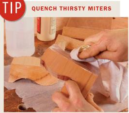
End grain soaks up glue quickly, drawing it from the surfaces and weakening the joint. The solution is to seal the end grain with an initial coat of glue, a process called "sizing." Let the glue absorb for a minute or two, then wipe it off with a rag moistened with water. Let the pieces dry completely before applying more glue and clamping them.
