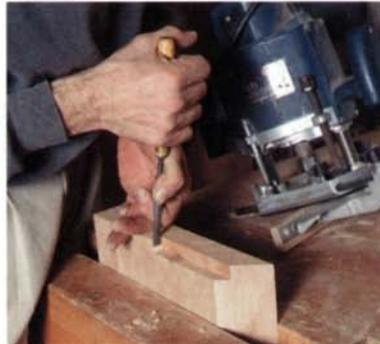
**Rout a stopped rabbet on the upper inside edge of each leg half.** Then square the end of the rabbet with a chisel.
