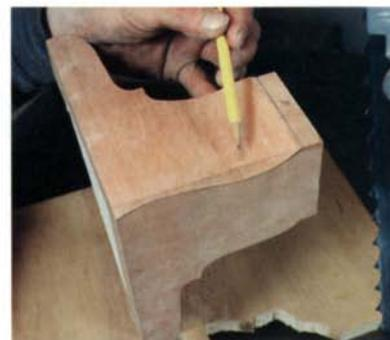
**Reposition the stock on the jig to cut the other face.** The glue line serves as the layout line because it follows the profile exactly.
