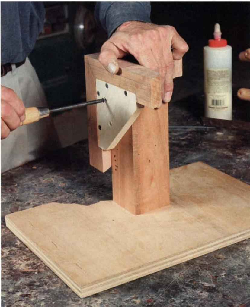
**Mount the blank to the jig by screwing through the corner block.** The jig consists of a post of solid wood screwed onto a piece of plywood large enough to balance the assembly while it's being bandsawed.
