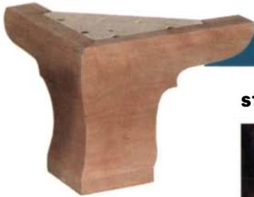
The foot derives its strength from an internal spline and a corner block. Although the corner block is screwed in place for the glue-up, to remain true to the period the author replaces the screws with antique nails before attaching the foot to the case.
