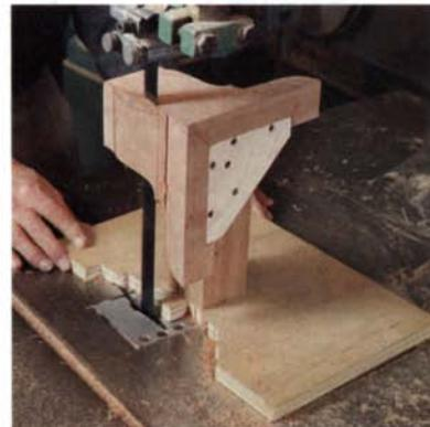
**Cut the outer profile.** The author nibbles away at the shape and cuts from both directions as needed.
