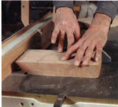
**Cut a slot for the spline on each face of the miter.** The author makes the cut on the tablesaw with the blade set at 45°.
