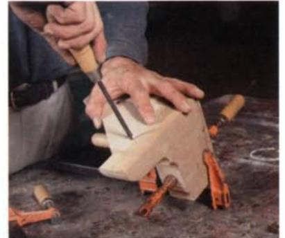
**After bandsawing the foot's inner profile, assemble the halves.** Use small bar clamps to close the joint, then strengthen it with a corner block glued and screwed into the rabbet.
