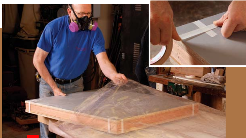
8 In the bag. Use masking tape to hold the top and bottom cauls in position (inset), then slide the sandwich into the vacuum bag.
