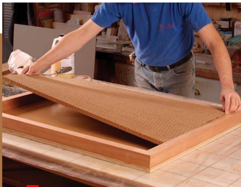
3 First layer of honeycomb. Place the first layer of honeycomb inside the frame. Press it firmly against the bottom skin and snug it into the corners.
