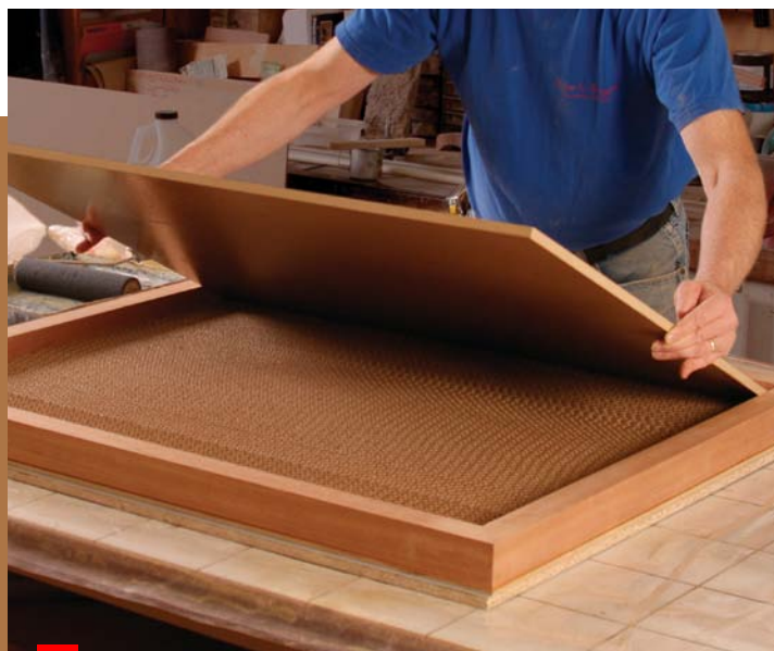
4 MDF is next. After rolling glue onto the bottom of the middle MDF panel, lower it into the frame. Press it down so it sits flat.
