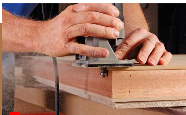
9 Trim the edges. After the assembly dries, trim the top and bottom skins flush with the wood frame. You now have a perfect substrate for veneer.
