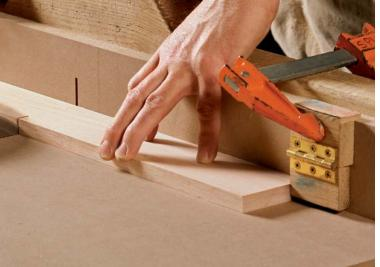
wide enough to accommodate a couple of clamps. Make the block thick enough (¾ in. to 1 in.) to provide a solid stopping surface. Relief cuts at the rear and bottom corners prevent dust buildup that could throw off a cut's accuracy.
