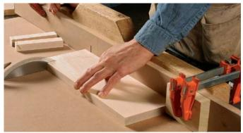
A few tips. Measure from the sled's kerf to locate the stop block, but elevate the ruler to avoid the relief cut under the block (above). Also, make sure the block is square to the sled's deck for accurate cuts in stock of any thickness.
