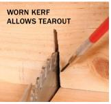
Over time, the blade opening becomes enlarged, leaving a gap around the blade. When this happens, the sled no longer supports the workpiece next to the cut. The result is tearout.
