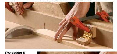
favorite. A hinge lets you swing the lower half out of the way when squaring the first end of a piece, then drop it into place for cutting to final length. A lip at the top references against the top edge of the sled's fence, squaring the block every time.
