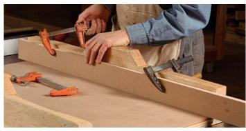
Fresh fence. Make the auxiliary fence from 3/4-in. MDF. Just clamp it on. Making the fence extra-long (as shown) isn't necessary, but it accommodates a stop block for longer workpieces.
