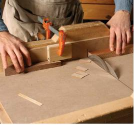
**Cut short pieces safely.** This sliding block controls the length of the offcuts, ensuring slices of equal thickness, but allowing them to fall freely away from the blade. Put the sliding block in place, and bump the workpiece against it (left). Then pull the block away before making the cut (right).
