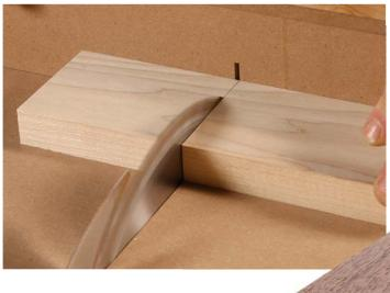
The payoff. The zeroclearance openings support the wood fibers where the blade exits the cut, helping eliminate tearout. As a bonus, you can trust the edge of the kerf when aligning your cuts.
