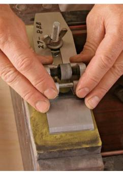
plastic also prevents the bolt head from creating a depression in the sharpening stone. Note: When you're setting the back-bevel angle, place the plastic under the bolt head so the angle doesn't change when you go to the stones.
