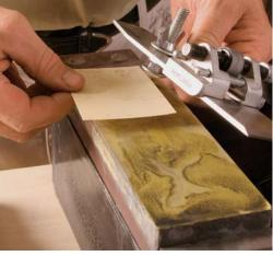
Short strokes on fine stones. Create the back-bevel on your two finest stones. Use short strokes and keep the bolt head on the plastic. Five or 10 strokes, and the blade is ready for the toughest woods.
