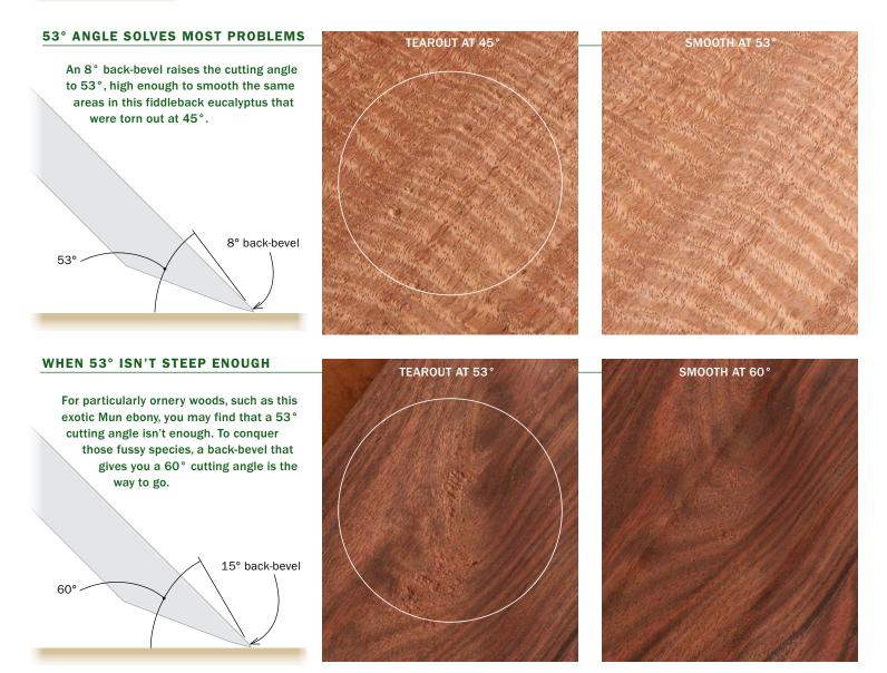
Since then, I keep two blades on hand: one with a back-bevel and one without. I use the standard blade almost all of the time. But when I notice that I'm getting tearout in challenging grain, I replace the standard blade with the back-beveled one.
