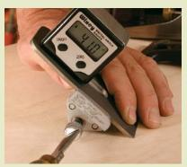
The cutting angle of a bevel-up plane is determined by adding bevel creates the bed angle of the tool and the bevel angle of the blade. Most bevel-up planes have a bed angle of 12° and a factoryground bevel of 25°, which produces a low cutting angle of 37°. So creating a higher angle is as easy as honing a steeper bevel on the front side-no back-bevel required. To get the 53° cutting angle, Gochnour adjusts his blade to hone the secondary bevel at 41° (left), then he sharpens the blade (below).
