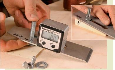
**Dial in the angle.** Slide the bolt, washer, and nut all the way to the back of the blade slot. Thread the nut up or down to get the back-bevel angle, in this case 8°. Gochnour uses a digital angle gauge, but a wedge block (inset) would work, too. The plastic shim that protects the sharpening stone in use (facing page) affects the angle, so place it under the bolt. Once the angle is set, let the glue dry and then secure the jig to the blade with the other washer and the wing nut (below).
