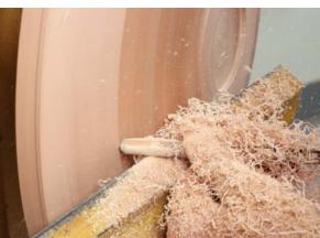
Scrape it. Use the burr on a round-nose scraper to clean up the surface prior to sanding.
