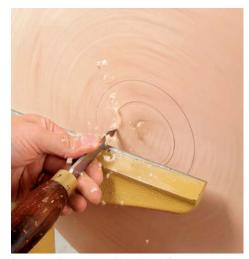
Lay out the recess. Use the calipers to mark the diameter of the recess on the spinning workpiece. Mark the outside of the foot, too, and then use a parting tool to cut the shoulder.
