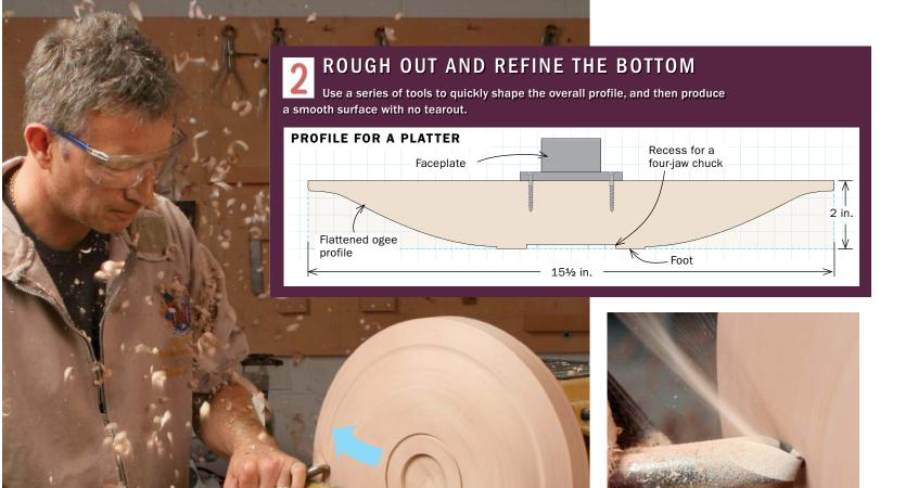
Rough it. When shaping the outside of the workpiece, cut from the center toward the edge, going with the wood fibers. Use the ¾-in. bowl gouge. The side bevels, or wings, on the gouge can be used to make light, shaving cuts to clean up the surface.
