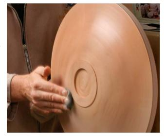
A flawless finish. Because you sealed the wood first, the subsequent oilbased finish leaves an even sheen.
