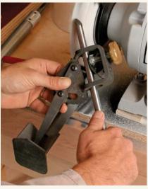
Set the base of the jig in the V-arm and swing the jig back and forth until the wings are fully shaped.
