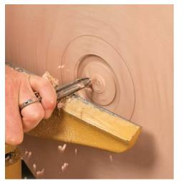
**Complete the recess.** Use the long-grind %-in. bowl gouge to remove the rest of the waste from the recess.
