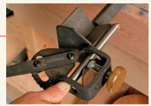
Place the gouge in the Vari-grind jig with its adjustable arm in the second stop from the bottom. Place the jig against the back of the V-arm support and extend the tip of the gouge until the base of the bevel is level with the front of the V.
