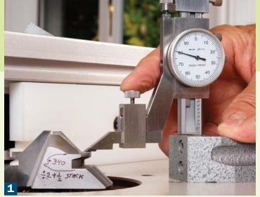
**Measure the upper cutter first.** Lower the probe onto the horizontal surface of the lock-miter bit's upper cutter. Note the highest whole number on the vertical beam (7) and add this to the number on the dial (80), to give 0.780 in. By the way, the overall bit height or location doesn't matter right now.
