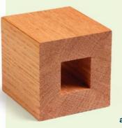
The 45° lock-miter joint combines the clean-flowing lines of a miter joint with a locking mechanism that both makes the joint stronger and prevents the parts from sliding around during gluing.
