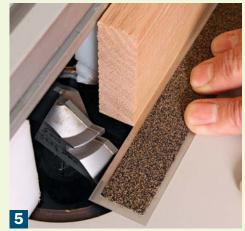
**Set the fence.** Place the stock vertically against the fence close to the bit. Hold a rule against it with a couple of inches in front of the bit. When the bottom 45° cutter just misses the rule, lock the fence.
