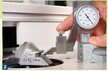
**Next, measure the lower cutter.** Place the probe on the lower lock cutter and note the measurement, in this case 0.440 in. Subtract the 0.440 in. from your upper cutter's measurement of 0.780 in. to obtain 0.340 in.—the distance between the upper and lower cutters. Now divide the 0.340 in. by 2 to give 0.170 in.
