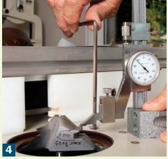
**Set the height.** Set the gauge to 0.588 in. and raise the bit until its upper horizontal cutter contacts the probe. The centers of the workpiece and the bit are now aligned. Later, write the formula on the bit to speed future setups.
