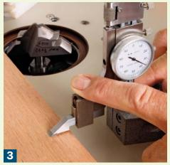
How thick is your stock? Lower the probe onto your stock to measure its thickness. In this case it is 0.836 in. or a shade under  $^{27/32}$  in. Divide this by 2 to give 0.418 in. Add 0.418 and 0.170 to get 0.588 in.
