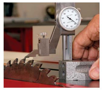
**Exact blade heights.** Very few tablesaws have a system to measure blade height, and using a rule or a combination square is not ideal. You can set the height gauge to the exact height you want the blade, and then raise the blade until the tip of a tooth just touches the probe. On a dado set, register the height of an inner chipper tooth, as they determine the core depth of the rabbet or dado, not the outside blades.
