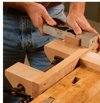
Tame your tenons. A shoulder plane can be used on its side (left) to trim a tenon’s cheeks. Used vertically (right), it can trim and square the tenon shoulders.
