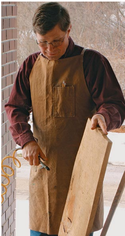
Compressed air removes the bulk of surface dirt. Clean boards outside, away from machinery, tools, and workbenches.
