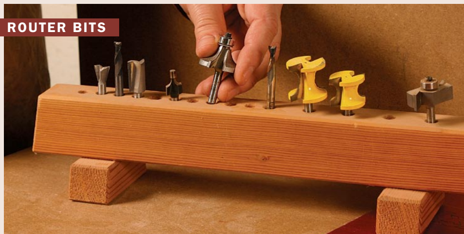
Make portable racks for your router bits. A small rack is portable and easy to make from scrap lumber.
