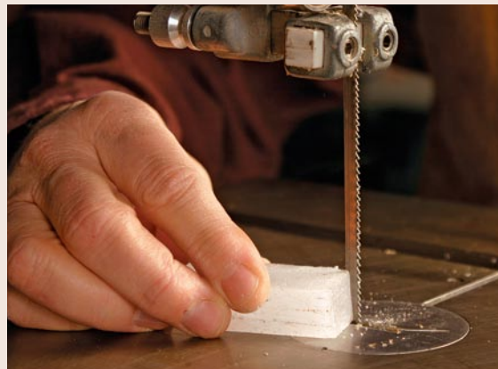
Wax bandsaw blades to reduce friction. With the blade running, hold a piece of paraffin wax on the table and against the blade.
