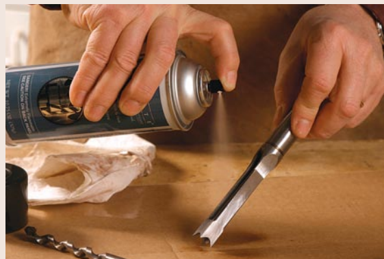
Apply a dry lubricant on chisel mortisers. The lubricant helps prevent buildup and keeps bits from dulling prematurely.
