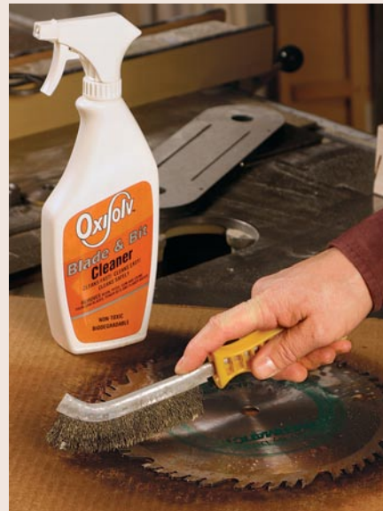
Use a blade-and-bit cleaner on tablesaw blades. Spray it on the buildup and let it sit before scrubbing with a brass brush.
