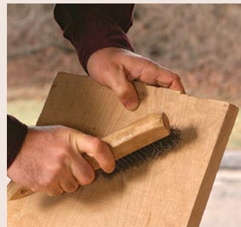
Use a wire brush to dislodge the rest. Scrub in the direction of the grain to remove debris.
