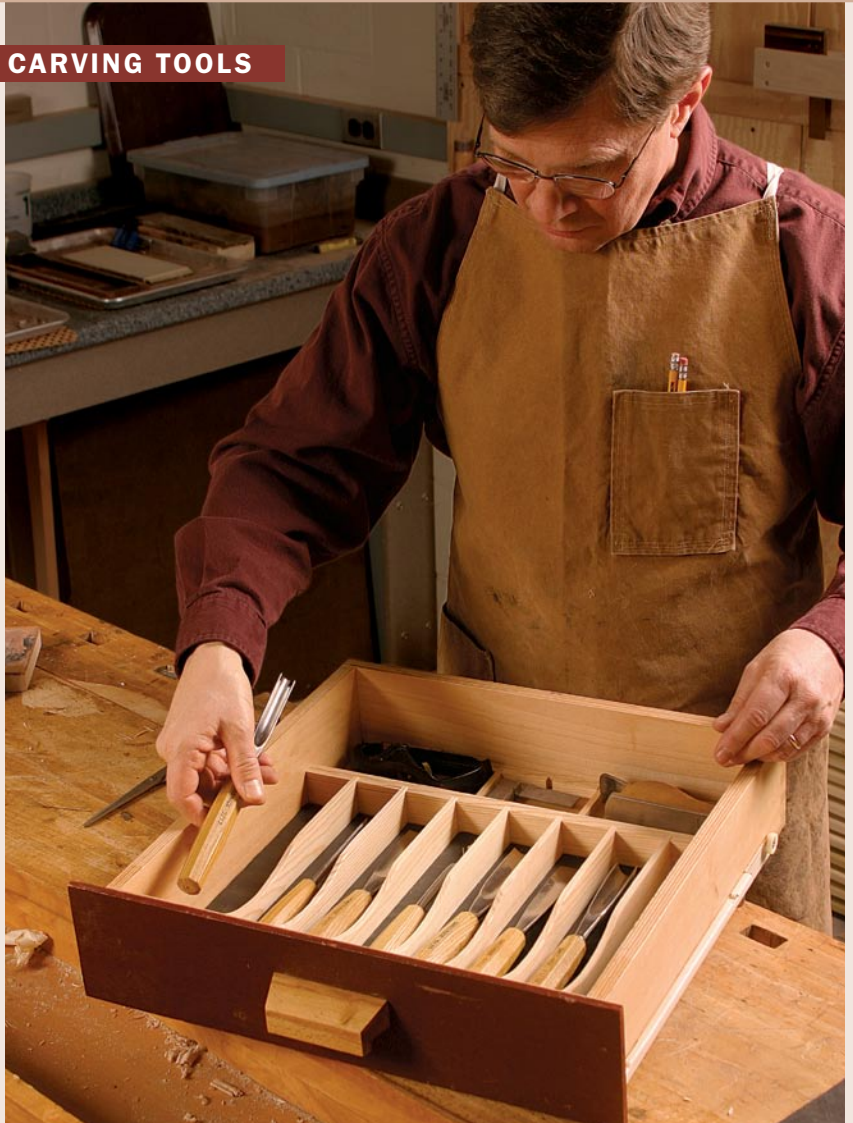
Lesser-used tools can be stored in drawers. Custom-made drawer dividers will help keep carving tools sharp.
