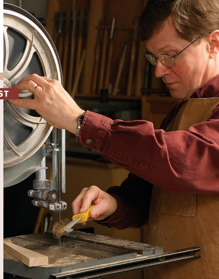
Clean bandsaw gullets. With the machine turned off, rotate the upper wheel by hand as you pass a brass brush over the blade.
