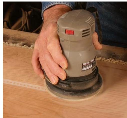
Sand away the tape. Use a random-orbit sander to remove the veneer tape and to prepare the surface for finishing.
