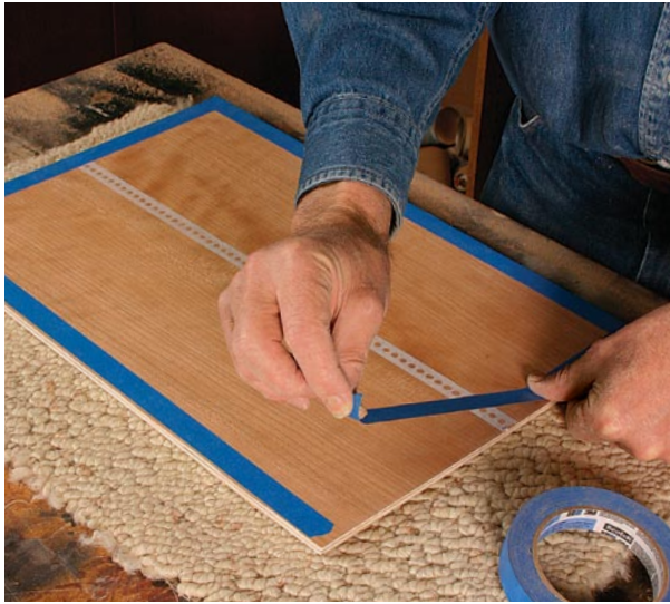
Tape tames tearout when cutting the panel. Apply masking tape to the back face along the line that will be cut on the tablesaw (above). Cut the panel to fit the frame with the show face up (above right).
