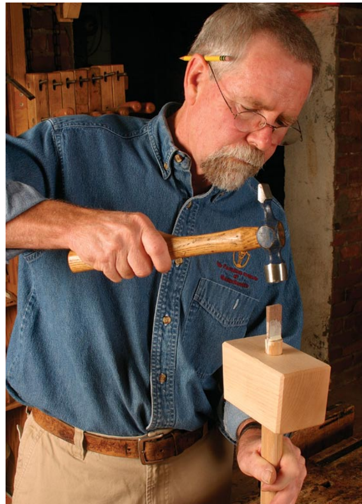
Drive the wedge until it stops. When the glue dries, use a handsaw and chisel to trim the handle and wedge flush with the top of the mallet.
