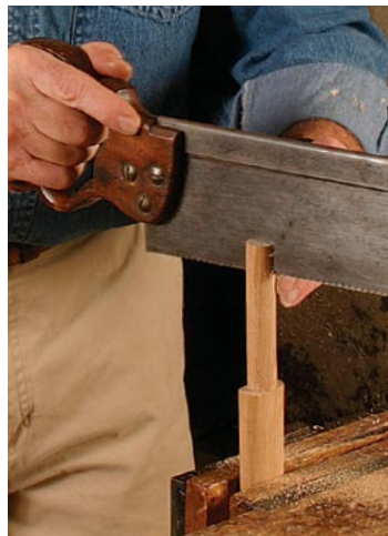
Finish shaping. Blend the contours and smooth the surface. Next, saw a kerf about 2 in. deep through the center of the tenon. The kerf should be parallel with the striking faces in the assembled mallet.
