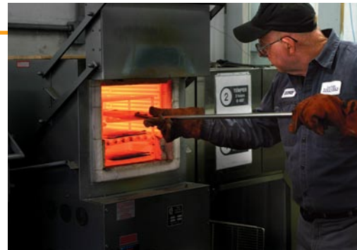
Fire and ice. To improve hardness, the steel plane blades are heated in an oven until red hot (top). Later, to improve wear-resistance, the blades are subjected to a Pluto-like temperature of minus 320°F (bottom).
