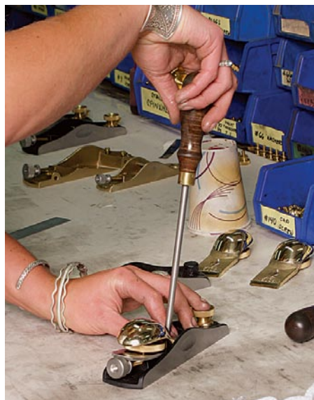
Putting things together. All the parts converge in the assembly department, where the planes are put together by hand.
