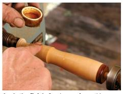
**Apply the finish.** Smalser prefers a thin wiping varnish formulated for gunstocks (Tru-Oil or Lin-Speed), rubbed out with paste wax and #0000 steel wool after curing.
