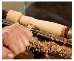
**Cut the handle to final shape.** Use the small gouge followed by a skew chisel for cleanup. This design relies on subtle curves for comfort.
