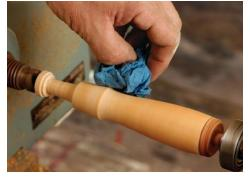
Raise the grain. Wipe the handle with a damp towel between each grit. The water swells and loosens the wood fibers in the scratches, so less work is required to sand them off.
