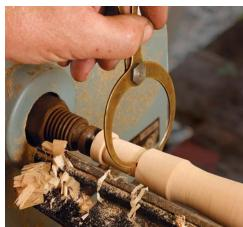
**Use an inside-outside caliper.** Transfer the inside diameter of the socket mouth to the tenon shoulder, checking progress as you cut the top of the tenon to size with a parting tool.
