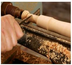
**Finish the taper.** Gauge the socket's depth and its diameter at the deep end. Use these measurements, and the parting tool, to cut the small end of the tenon to size. Finish the taper by pulling a small skew from the tenon shoulder to the pointed end. Leave the tenon slightly oversize for hand-fitting later.
