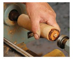
**Start by turning a stub tenon.** Smalser uses a parting tool to form the tenon, and then glues leather washers over it to create a durable striking surface.
