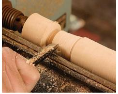
**Establish the tenon shoulder.** Use the parting tool to mark the start of the tenon that fits in the chisel socket, then shape the adjacent tapered section with a small gouge.
