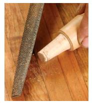
An age-old fitting trick. After securing the blade in a vise, insert the tenon firmly and twist it a full revolution. A dirty socket will leave dark patches on the high spots; file these away using a fine rasp. Repeat until you have full wood-to-metal contact for a perfect fit.
