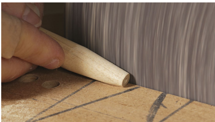
Sand to shape. Thibodeau tapers the front end to create a comfortable grip, then rounds over the back end.
