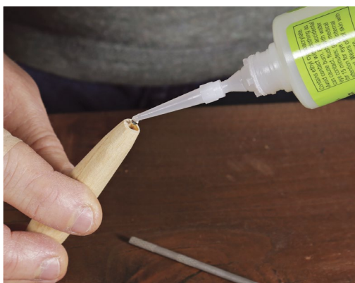
Drop in the glue. All it takes is a few drops, guided into the hole with the help of a needle tip (left). Slide in the chisel, pushing it as far as it will go with hand pressure (right). While holding the chisel up off the bench, rap it firmly on the end of the handle (far right). Repeat until the blade bottoms out in the hole.
