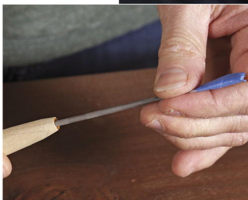
Drop in the glue. All it takes is a few drops, guided into the hole with the help of a needle tip (left). Slide in the chisel, pushing it as far as it will go with hand pressure (right). While holding the chisel up off the bench, rap it firmly on the end of the handle (far right). Repeat until the blade bottoms out in the hole.
