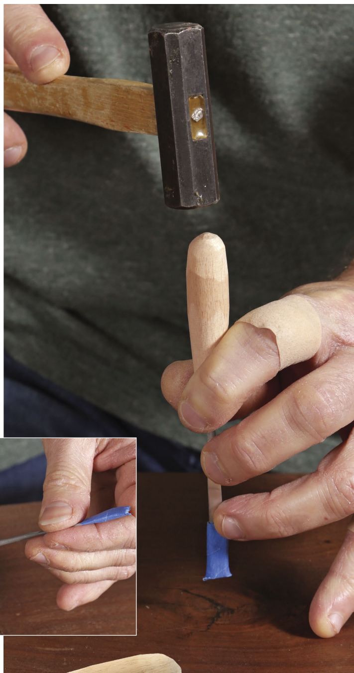
Drop in the glue. All it takes is a few drops, guided into the hole with the help of a needle tip (left). Slide in the chisel, pushing it as far as it will go with hand pressure (right). While holding the chisel up off the bench, rap it firmly on the end of the handle (far right). Repeat until the blade bottoms out in the hole.
