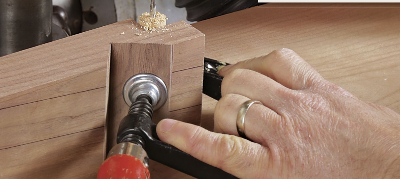
Handle gets a hole. Clamp the handle into a notched block so that it doesn't move while being drilled.
