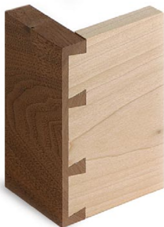
VARIABLY SPACED HALF-BLIND DOVETAILS (VHB)
