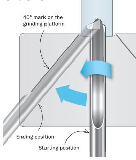
will help you get a consistent side-to-side sweep. Make a template from scrapwood cut to the same size as the platform. Mark the guidelines with an indelible marker.
