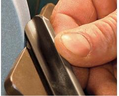
**Start with the flute facing up and the tool centered on the grinder platform.** Sweep the gouge in an arc to the left, simultaneously rolling the tool so that the gouge faces left. End at the 40° guideline on the grinder platform. Then sweep and roll the gouge to the right.
