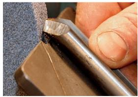
**Grind the nose to check the angle.** Test the platform angle by lightly grinding the nose of the gouge, then checking the result with a protractor or angle gauge.
