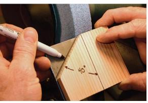
**Make a template.** Cut one corner of a piece of scrap at a 40° angle and use it to mark the grinder platform.
