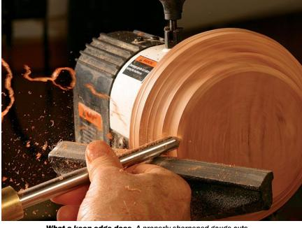
What a keen edge does. A properly sharpened gouge cuts efficiently and doesn't need a lot of muscle to do its work.
