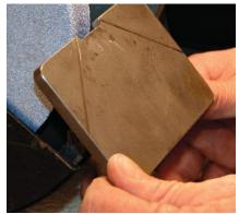
**Angle the grinder platform.** Use trial and error to set the platform at a 40° angle (or close to it), which will be the bevel angle on the gouge.
