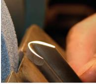
**Start a new cutting edge.** With the gouge's flute facing down, grind away the cutting edge. The resulting thin face creates a guide for the last stage of sharpening.
