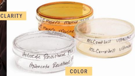
Waterborne finishes can add color. Some of the finishes, such as Hydrocote Resisthane Plus, dried clear. Others, such as M.L. Campbell Ultrastar, added a touch of yellow, while J.E. Moser's Marine Shield was dark yellow.
