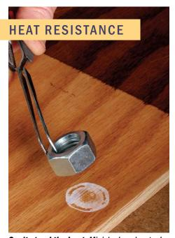
Can't stand the heat. Minick placed a steel nut, heated in boiling water, on each test panel and evaluated the results after 24 hours. Most finishes survived unscathed; Moser's Simple Success simply failed.
