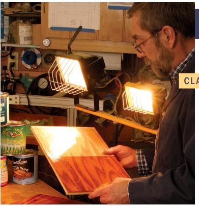
A clear finish. Each panel was examined under a halogen light for color and clarity. Only a few finishes exhibited the bluish cast that was once the trademark of waterborne finishes.
