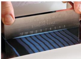
See how they run. A notched drawdown bar applied strips of finish ranging from 3 mils to 12 mils in thickness. The test card was then hung up to dry and the thickest line that didn't sag or run was recorded. This gives an indication of how forgiving a finish will be if too thick a coat is applied to a vertical surface.
