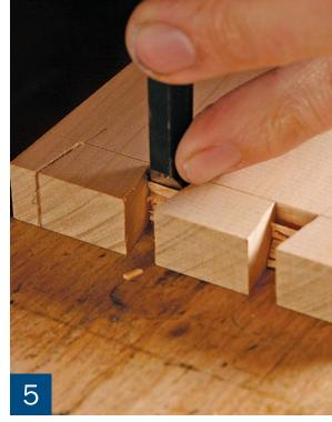
**Pare to the layout line.** Afterward, use a small square to check that the sawn and chiseled surfaces are square to the face of the board. This helps ensure that the finished joint will go together tightly.
