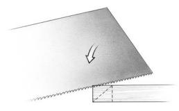
2. Steepen the angle to vertical as you finish the cut, taking care not to lift the saw out of the kerf or overcut the scribed line.
