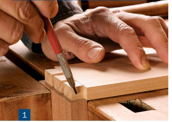
**Trace the tails to lay out the pins.** Place the drawer front vertically in a vise. Hold the drawer side firmly in place while tracing the outline of the tails on the end grain. Swensson uses a pencil sharpened to a chisel edge on a sanding block.
