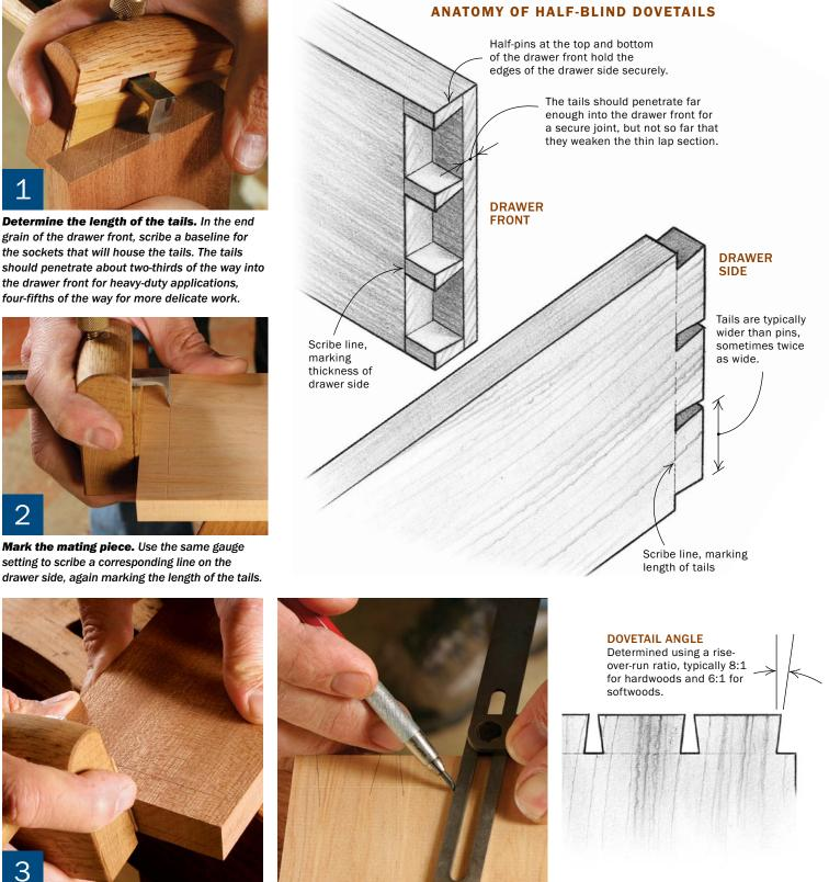
Set the socket depth. On the inside face of the drawer front, scribe a line to match the thickness of the drawer side, plus 1/32 in. or so.
