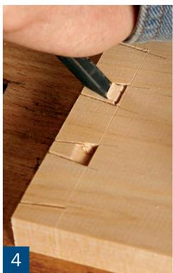
**Start chopping out the waste.** Make a vertical cut about <sup>1</sup>/<sub>32</sub> in. on the waste side of the scribed line. If you start in the scribed line, the natural cutting action of the chisel will push it past the line.
