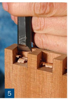
Clean up and check the fit. Pare to the layout lines (above), again checking the chiseled and sawn surfaces for square. A firm rap with the fist should be enough to get the joint started (right).
