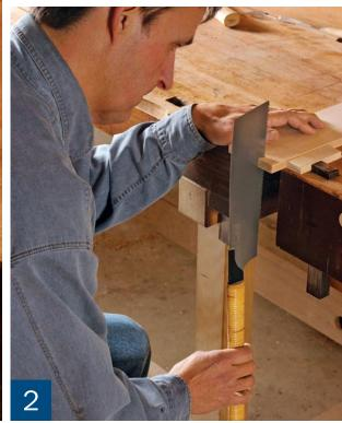
**Start the saw at a low angle.** This helps establish the kerf over the full length of the cut. Swensson secures the drawer side flat on the benchtop with the end grain facing him.
