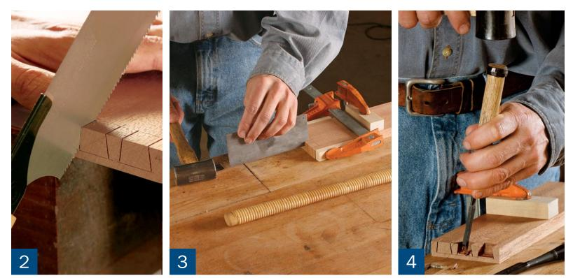
**Start the kerf with a saw.** Again, start at a shallow angle and steadily steepen the cut. Make sure that the saw arrives at both corners simultaneously.
