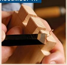
A chamfer eases the fit. Cut a narrow chamfer on the mating edges of the pins and tails. This protects the corners from crushing or tearing when fitting the joint.
