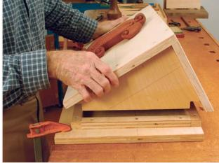
An angled easel places workpieces at a more comfortable height and angle. The four bottom corners are notched to fit within the fences on the base (above), and the easel is held in place by its own weight. Lips on the top outside edges allow for clamps to hold some workpieces in place (right); others can be secured with screws from behind.
