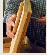
When carving blanks with flat backs, screw the blank to the base of the carving station (above) to hold it in place. Take care to locate screws where they will not damage carving tools (right).
