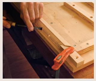
A fence set back from the edge of the base leaves a perfect space to support long pieces of molding, which Wilbur clamps in place using scraps of wood cut to the shape of the molding and cushioned with foam rubber padding (right). Shorter, mitered pieces can be locked in place with mitered cleats that are screwed or clamped to the base (above).
