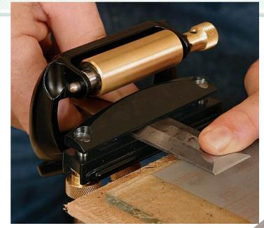
**Remove the burr on the back.** To remove the burr that forms on the back of the bevel edge, the final step is to place the back of the chisel on the 0.3-micron paper and slide it back and forth until the burr breaks off.
