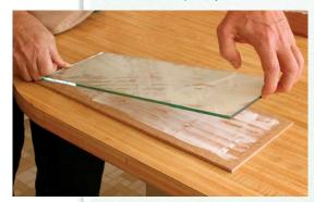
Strengthen the glass with a backer board. The glass becomes less fragile when glued to a piece of hardboard.
