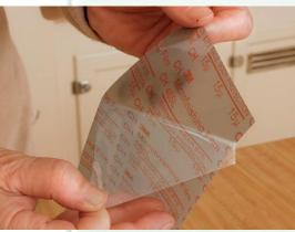
Peel away the plastic backing on the sandpaper. Although the paper is selfadhesive, apply a thin coat of soapy water to the glass. This will make it easier to position the paper.
