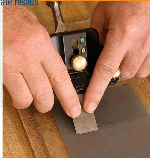
uniform in size. That means you are less likely to get unwanted deeper scratches from an occasional oversized grit in your paper. Plus, because the sandpaper mounts firmly on glass, the abrasive stays flat. I use three grits—15 micron, 5 micron, and 0.3 micron—one for each piece of glass.
