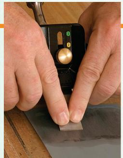
**Continue through the grits.** With the jig set to  $31^{\circ}$ , Beach hones the second microbevel on the 5-micron paper. He then raises the angle to  $32^{\circ}$  for the final passes on the 0.3-micron paper.
