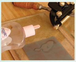
**Start with 15-micron paper.** Add a little baby oil or mineral oil to help float away the steel filings. Set the jig at 30° and roll it back and forth, keeping the wheel off the sandpaper. It takes a minute or less to establish the first microbevel.
