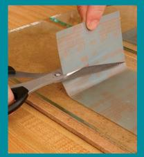
When a section of paper finally wears out, simply peel up the worn section and cut it off with scissors. Any residue from the adhesive backing can be removed from the glass using baby oil or mineral oil and a soft cloth.
