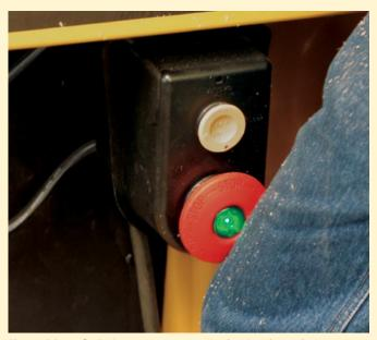
**Kneeable switch.** In an emergency, the jumbo-size switch on the Powermatic PM2000 can be easily reached with a knee. The green-glowing center lets you know that the saw is powered up.
