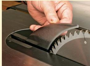
Riving knife reduces the chance of kickback. A riving knife, found on the Laguna TS-10, Powermatic PM2000, and SawStop 31230, helps prevent the workpiece from pivoting onto the rear of the sawblade during a cut.
