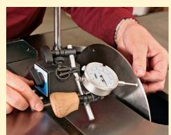
Blade/miter slot parallelism. A 10-in.dia. flat plate and dial indicator were used to find out if the sawblade is parallel to the mitergauge slot when the blade is at 90° (shown) and 45°. Misalignment can be corrected.
