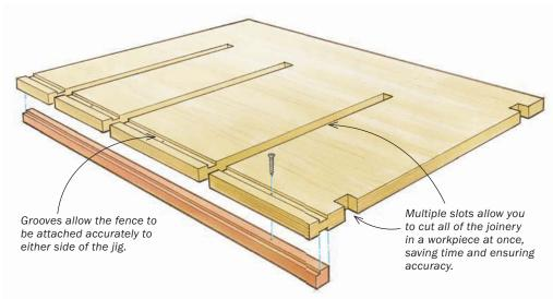
Dadoes and dovetails. This jig lets Miller cut a combination of long, shallow dadoes and short dovetail slots in three different spots on a solidwood case side.
