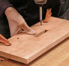
**Add the fence.** Make the fence wide enough to extend from the edge of the template to the edge of the workpiece (don't forget the offset). Clamp it in place, feeling with your fingers to keep the outside edges flush (left). Then flip it over and drive screws (right).
