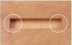
**Set up for mortising.** Bring the edge of the template to the edge of the workpiece, then extend the bit down to a line that represents the desired mortise depth and lock it there (top). You only have to mark the ends of the mortise to locate the jig accurately on the workpiece (above).
