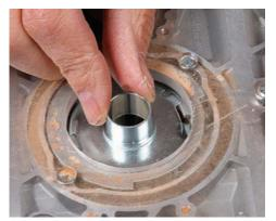
Attachment varies by router. The most common style is the Porter-Cable, which is held in the base of the router or an adapter by a threaded ring (left). Bosch's bushings are even easier to use, dropping into a spring-loaded holder (right).
