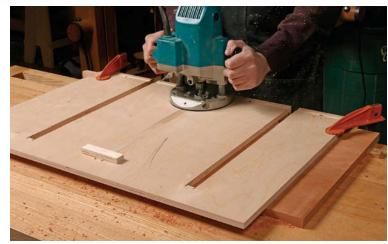
indication of where to align the jig. Just line up the cut in the fence with your layout marks.
