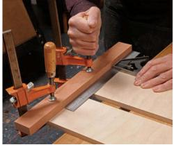
Cut the slot and add a fence. Make long cuts, turning off the saw at the end of each cut, and then remove the waste with a jigsaw. Clamp the fence square to the slot and screw it in place.
