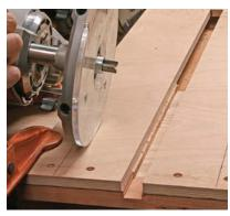
Start with a straight bit and follow with a dovetail. Plow out a dado just narrower than the narrow part of the dovetail you'll be cutting (above). Follow with the dovetail bit. It helps to have a second router set up with the dovetail bit, so you don't have to change bits and lose your depth settings for each (right).
