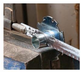
Most bushings need a trim. For the bushing to work with thin templates. vou should saw off some of the excess length. Leave 1/4 in. to 3/8 in. to engage the template.
