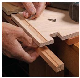
**Make it reversible.** The fence on this big jig has a shallow tongue that fits into matching grooves on either side, so it can be flipped for two opposite sides of a case.
