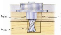
The 1/8-in. slot is wider than the bushing in this case, in order to let a ½-in, bit cut a 3/4-in.-wide dado.
