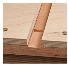
Up and back. Use the notch in the fence to line up the jig with your layout marks (above). Push the router up the left side of the jig and then pull it back along the right side to keep the bushing tight to the walls of the slot on both sides (right). Square the ends of a stopped dado with a chisel.
