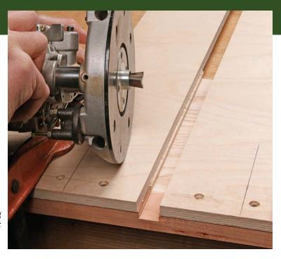
is set, push the spacer strip out of the jig. Then joint and/or plane the template to make it flat.
