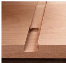
Another handy stop. After plowing the dado, drop in a strip to set the length of the sliding dovetail (left). This stop goes in and out easily between dadoing and dovetailing. The jig ensures that the sliding dovetail is perfectly centered on the dado, and accurate in length (above).
