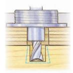
Use a straight bit to remove most of the waste before dovetailing.
