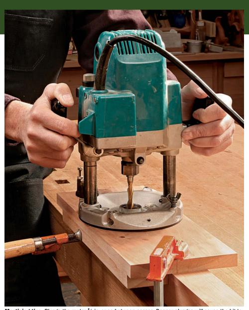
**Mortising tips.** Plunge the router ½ in. or so between passes. Deeper plunges will cause the bit to wobble slightly and cut an oversize mortise. Also, be sure to keep the router oriented the same way throughout the process. If the bushing is slightly out of line with the bit, the offset will vary when you twist the router, changing the path of the cut.
