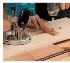
Stops are easy to add. For stopped dadoes, screw down a block to stop the router in the right spot.
