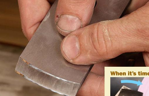
Even shine along the edge. You are done honing when there is an even polish along both the top and bottom of the bevel. At that point, remove the burr on the back of the blade.
