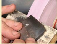
Hollow-grind the bevel. Begin with one corner of the blade in contact with the wheel (left), and then pivot the blade so that the bevel runs smoothly across the wheel, stopping when you reach the other corner (right).
