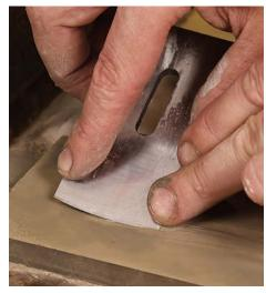
Honing with a swing. The action is similar to the pivot used at the grinder. Start at one corner (left), and pivot your wrist as you move the blade down the length of the stone. You should be honing the blade's trailing corner when you reach the end of the stone (right).
