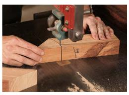
Clear the throat. After cutting the back of the throat, or bed, at 45°, cut the front side. Kellogg prefers a sweeping arc here to a straight cut.
