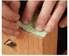
Lay out the curve. After aligning the template with the centerline, trace the curve onto the end grain. Repeat at the other end.
