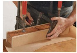
Glue it back together. Clamp the plane's center to the bench to keep it and the sides in alignment on the bottom. A bit of paper prevents the plane from getting stuck to the bench.
