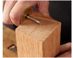
Mark a centerline. Scribe centerlines on both ends of the plane body, and then connect them along the length of the sole with a pencil line.
