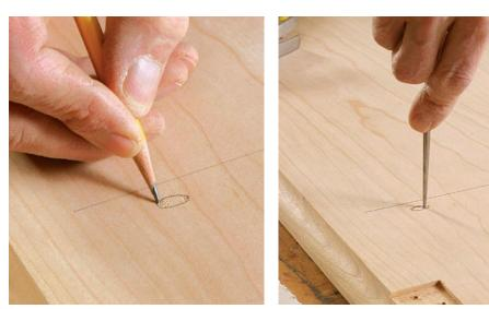
**Outline the elongated holes and locate the position of the outside screws.** With the points made by the scratch awl as a guide, use a pencil to scribe the elongated shape. If you anticipate the top is likely to expand, locate the pilot hole near the inside end of the elongated hole. If the top is expected to shrink, put the pilot hole near the outside end.
