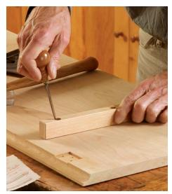
**Mark the hole locations.** Position the cleat on the underside of the top and mark the center of the middle hole. Make a series of points with a scratch awl to mark the elongated holes.
