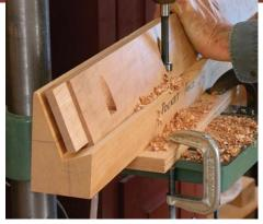
Jig simplifies pocket-hole drilling. A shopmade drill-press jig holds the apron at a suitable angle for drilling the pocket holes with a Forstner bit (above). A screw driven through an oversize shank hole in the pocket joins the top to the apron (right) while allowing the top to expand and contract.
