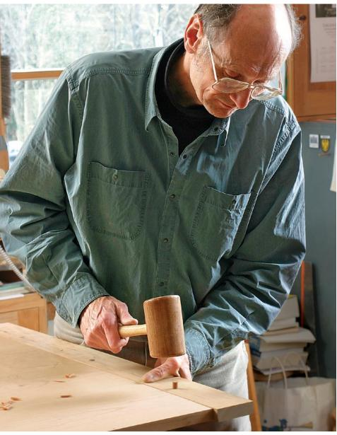
**Drive the pins.** Reassemble the breadboard ends after adding glue to the center tenon and mortise. Then add a thin coat of glue to each pin and drive them home. Trim the ends flush with the table.
