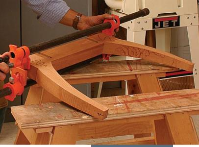
Assemble the leg frames. Cut the dovetail grooves in the leg rails, then join the leg rails to the legs (above). The horns prove handy here, as they provide purchase for the clamp jaws. Trim the horns after the glue dries (left).
