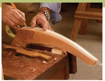
Fair the leg curves and mark the centerline. The bandsaw leaves the legs with a rough surface, so Rodriguez starts the shaping process by smoothing the front of each leg and marking a centerline (above) with a strip of tape serving as a flexible straightedge.
