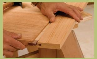
An easy technique for breadboard ends. A long mahogany spline (above), capped on each end with a short piece of walnut, is glued into a groove on each end of the top. On the breadboard-end groove, apply glue on only about 12 in. at the midpoint. A couple of pipe clamps (right) apply pressure to the joint connecting the top and breadboard ends.
