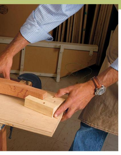
**Taper the legs.** A thickness planer and two jigs are used to taper the sides of the legs (left). With a leg in one of the jigs, taper the first side by elevating the bottom end of the leg % in. Then, transfer the leg to the second jig and taper the second side by raising the leg ¾ in.
