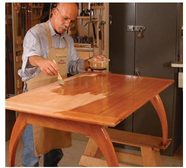
Mount the top and apply the finish. After attaching the top to the base, finish the table. A few coats of Waterlox Original, followed by a coat of paste wax, complete the project.
