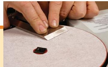
**Unmatched at flattening and lapping backs.** The foot switch and slow speed make the process easy to control, and the sandpaper quickly produces a mirror polish.
