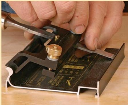
**Setup is quick and precise.** A clever registration jig sets the projection of the tool for various angles, and the tool holder keeps the blade square and level.
