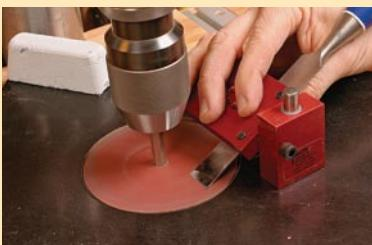
**Tool holder requires trial and error.** To adjust it, the holder must be lifted off the guide post.
