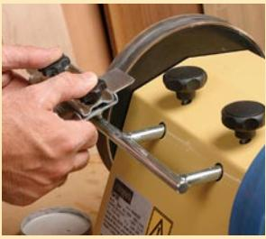
**Rougher grinding means slower honing.** Even when graded to its finest grit, the Scheppach's grinding wheel (top) leaves deeper scratches than the Tormek's does, which means more time at the honing wheel (bottom).
