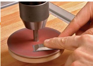
**Fast but inaccurate.** Runout in the thin aluminum platters creates rounded surfaces when lapping and grinding.
