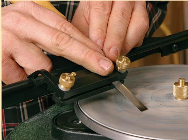
**The work goes quickly.** The speed of the platters makes for rapid cutting action, while the tool holder rides on a level rest for precise results.
