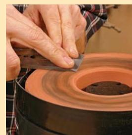
**Lapping is effective but inconvenient.** You'll either have to remove the tool rest or lower the splash guard, sending water flying.
