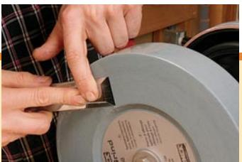
Flattening is easy on the side of the wheel. But lapping is done on the leather wheel, and requires careful technique to avoid rounding the back.
