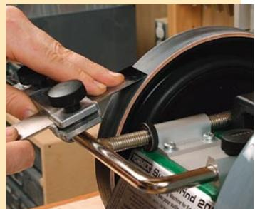
Charge the leather wheel with honing compound. Then switch over the tool rest, or do the honing freehand.
