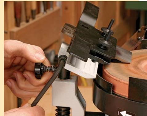
**First-time setup is fussy.** At least four adjustments are needed to set up the tool rest for sharpening.
