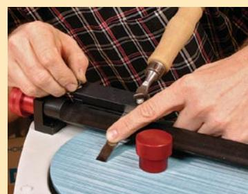
**The tool clamp could be better.** You must eyeball the angle to determine blade extension, and use a small square to ensure the blade is 90° to the clamp.
