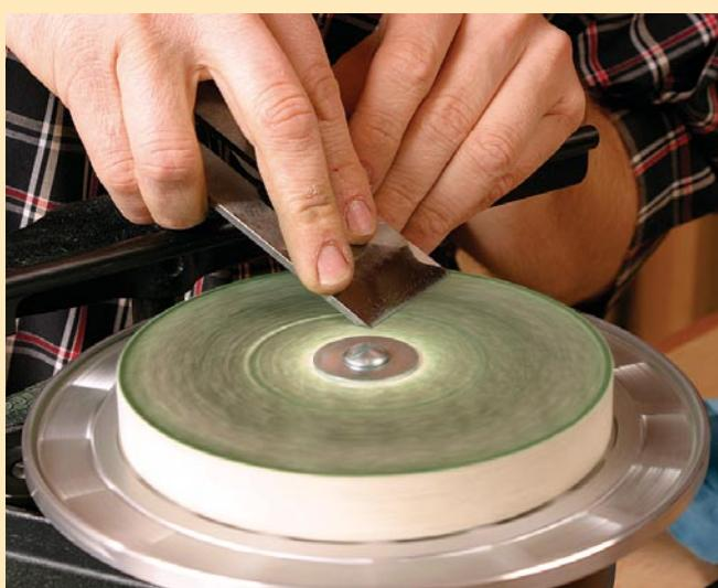
**Use the felt wheel for truly sharp edges.** This accessory wheel is charged with buffering compound and used freehand to bring backs and bevels quickly to a mirror polish.
