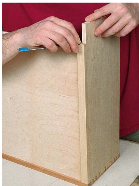
The drawer side is set in from the bottom runners and the sides of the drawer front (above). When laying out the half-blind pins, set a marking gauge about \frac{3}{16} in. heavier than the thickness of the drawer sides.
