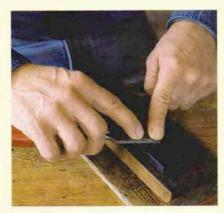
First flatten the tool's back. At least the first 34 in., and preferably the first 1 in. to 2 in., of the chisel's back should be perfectly flat. The back guides and controls the cut and ensures a fine edge.
