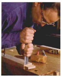
Chop, then pare. Lightly chopping all the way around defines the shoulder of a tenon (left) before a final paring with hand power (above).
