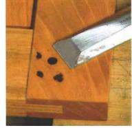
Paring pegs. A chisel with a flat back offers more control than a plane and is neater than a sander when leveling a pin.
