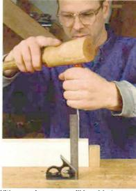
**The right angle for chopping.** With experience you will be able to hold the chisel at the correct angle merely by sighting across and down it (left). A square set on end acts as a guide when squaring up the end of a mortise (right).
