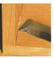
Clean up glue squeeze-out. A scraper works best for large areas, but for small areas a chisel offers more control.
