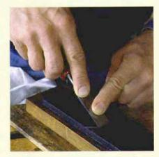
Grind and hone. After hollow-grinding a 25° bevel on the grinder, the author hones the bevel on a medium and then a fine oilstone. The author guides the chisel freehand, but a honing guide can help until you master the technique.
