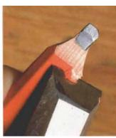
Handy pencil sharpener. A test of a chisel's edge is how fine a point you can put on a pencil.
