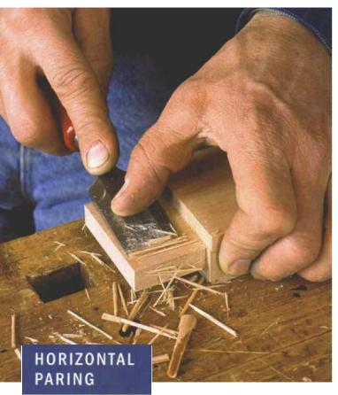
When cutting horizontally, the smoothest cuts are made with a slight shearing action, cutting both forward and sideways. The need for a perfectly flat chisel back is apparent when fitting a tenon.
