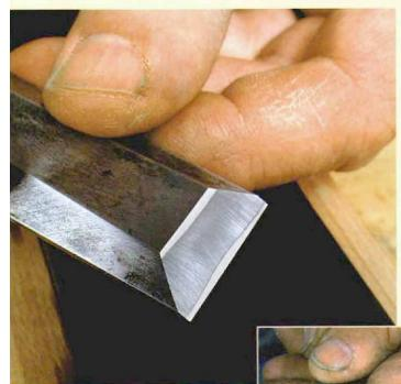
Ready to cut. The tuned chisel should be flat on the back and have a narrow band of honed steel along the cutting edge, with a slightly concave ground surface just behind. If you can leave a clean cut on pine end grain, your chisel is ready for action.
