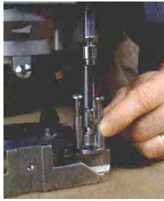
Three-step turret stop. The Festool has a turret stop with three adjustable steps.
