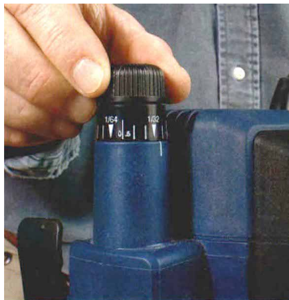
Fine-tune the depth of cut by turning a knob or dial. The Bosch, DeWalt and Festool allow micro-adjustments immediately after the housing has been plunged.
