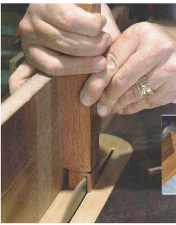
A higher fence for safety and stability. The extra height of the auxiliary fence provides a firm surface to press the workpiece against and helps keep hands away from the blade. Using scraps for testing the fit, make sure the two outside cheeks fit snugly into a mortise before proceeding with the cuts for the inside cheeks.
