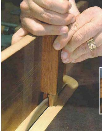
Almost there. Tweaking the final fit requires frequent checks with the set-up scraps before you can complete the final cuts on the workpieces. A snugly fit joint will go together smoothly with moderate hand pressure.
