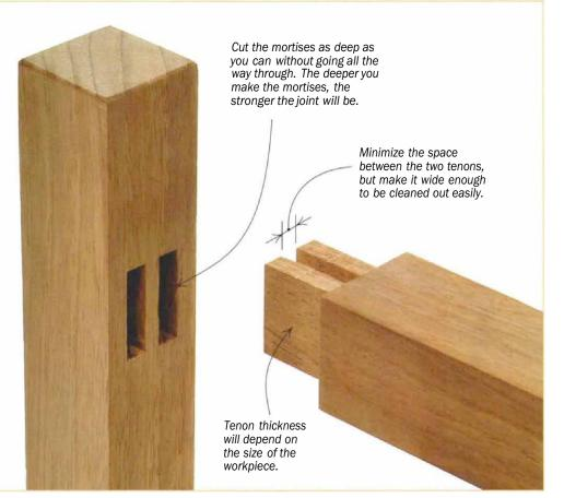
sible to maintain a strong joint. At this stage, having in hand a good sketch of the joinery detail is especially helpful.
