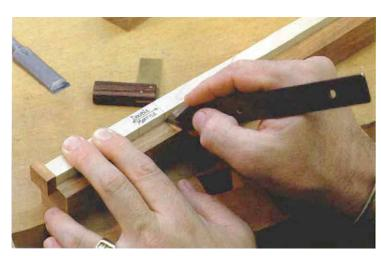
Tools for multiple marking. A story stick and a marking knife add accuracy and reliability to a repetitive process.
