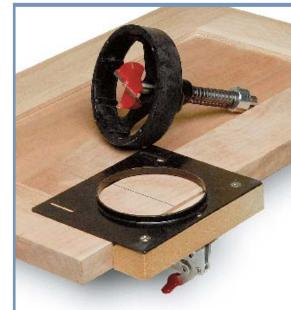
This jig has two main parts: a template (a steel base with a hardwood fence) and a plastic housing that accepts the built-in Forstner bit. The fence maintains an accurate backset. And clamping the jig is quick and easy. The Jig-It doesn't have guide holes for drilling the pilot holes for the mounting screws.
