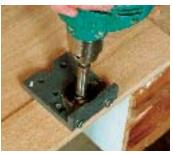
Start drilling. The hole in the jig acts as a bushing, keeping the Forstner bit contained and preventing it from skittering around as the cut starts.
