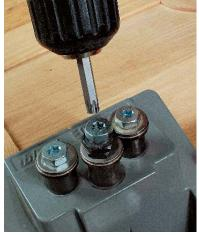
Drilling the cup hole and two pilot holes is as easy as one, two, three. One, insert the driver bit in the cap screw on the end of the 35mm Forstner bit and drill the hole; two, move the driver bit to a pilot-hole bit and drill; and three, repeat for the final pilot hole.
