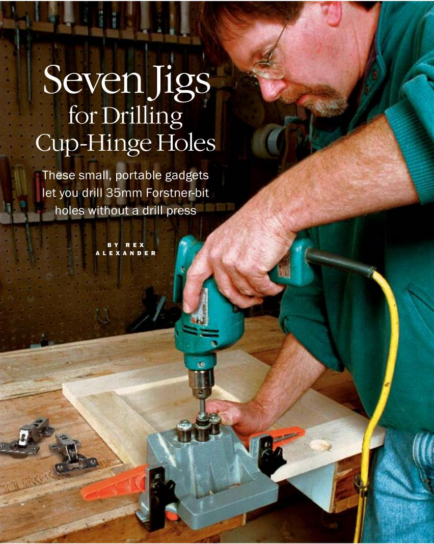
designated jig just to drill a hole? If you have cup hinges to mount, the answer just might be yes, because to make the hinge both strong and easy to install, the cup is designed to fit snugly into a 35mm hole bored in a cabinet door. A cup hinge installed in a sloppy hole won't enjoy full strength. So you want the hole to be a good one. That's exactly what these jigs promise to help you do.
