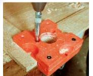
**Drilling the mounting holes.** A self-centering bit is used to drill the pilot holes for the mounting screws. The jig has four pairs of predrilled holes for the bit.
