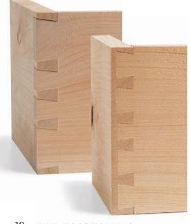
Promise to make flawless dovetails quickly and easily. To help you pick the best one, *Fine Woodworking* asked me to test the field. There's a pile of dovetail jigs on the market, so we tested only the ones that can do both half-blinds and through-dovetails, as both are essential for furniture making.
