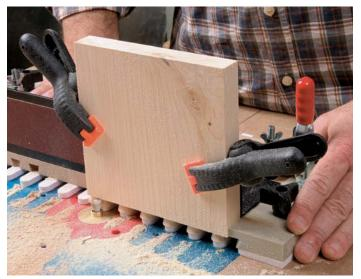
**Disposable stops.** You rout into the plastic end blocks for many joints, making them increasingly difficult to use for later tasks.
