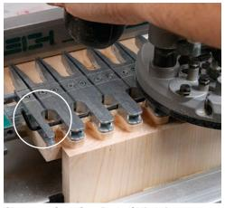
**Clever engineering.** For half-blinds in one pass, a rod slides through the template fingers to stop the bushing's rearward travel in the right spot.
