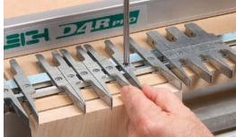
Magic fingers. All you need is a center mark to design the array of pins (left). You can trust your eyes from there, and even if the symmetry is off, the design of the template ensures a perfect match between pins and tails when you flip it (below).
