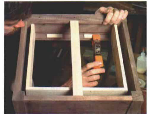
Drawer stops are glued to the lower rail. To position the stops, remove the drawer bottom, replace the drawer and position the stops against the inside edge of the drawer front.
