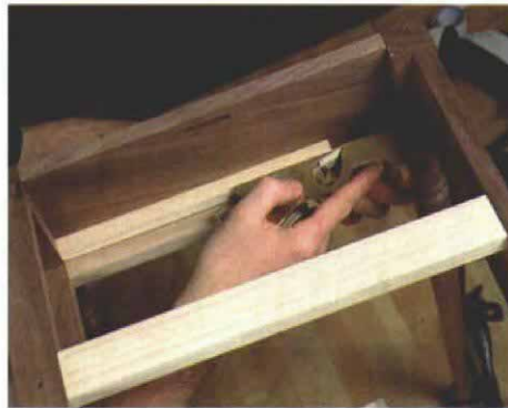
The drawer guide is notched and shorter than the runner. When it comes time to fit a drawer, plane only the guides, not the sides of the drawer.
