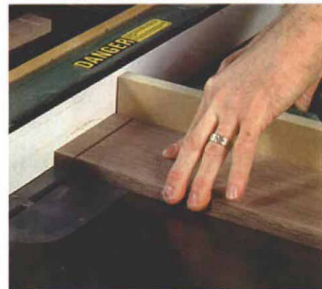
Raise the blade to \frac{3}{8} in. Cut the shoulders on the faces of all the aprons. The stock left between the kerfs should be \frac{3}{4} in. thick.
