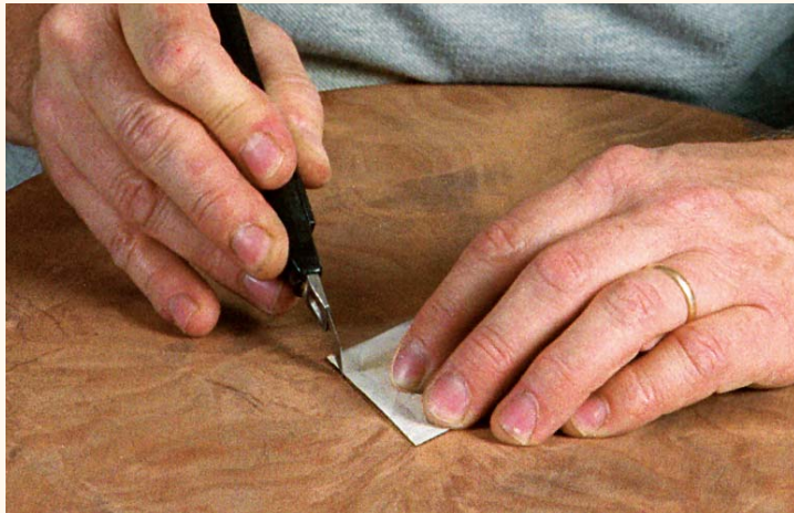
2 Cut around the inlay. Using a very sharp hobby knife, cut into the tabletop using the edge of the inlay as a guide. Keep the blade at a right angle to the tabletop to achieve a straight incision.
