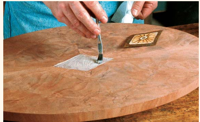
5 Glue the inlay. A generous coating of yellow glue lessens the chance of the inlay blistering. An X marked on the inlay and the veneer ensures consistent orientation.
