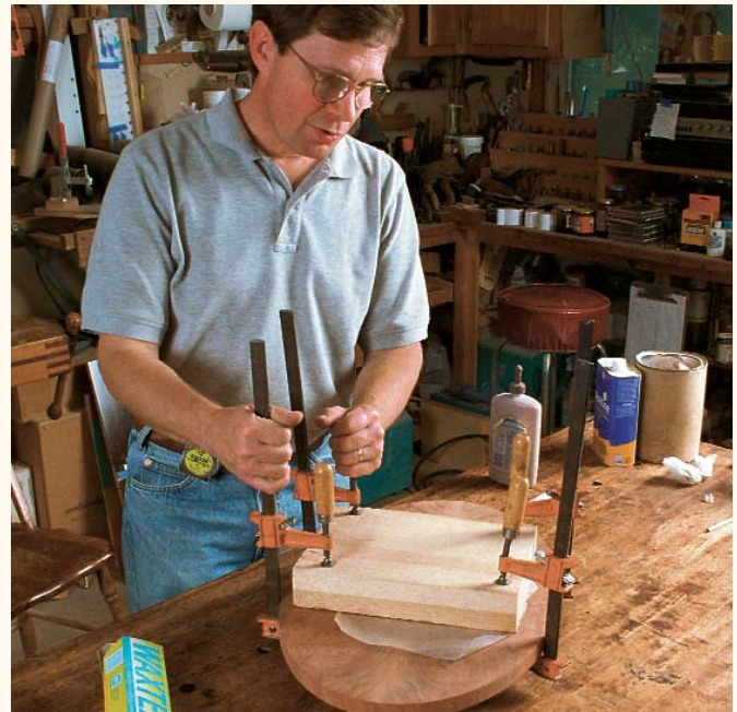
6 Clamp the inlay. A layer of wax paper between a sturdy caul and the inlay prevents squeezed-out glue from bonding the two together. Leave the clamps on overnight to ensure a tight bond.
