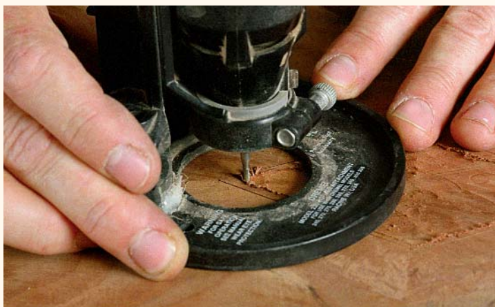
3 Rout away the waste. With a Dremel attached to a router-type base and a 1/8-in. straight bit, cut as close to the knife cut as you are comfortable with.
