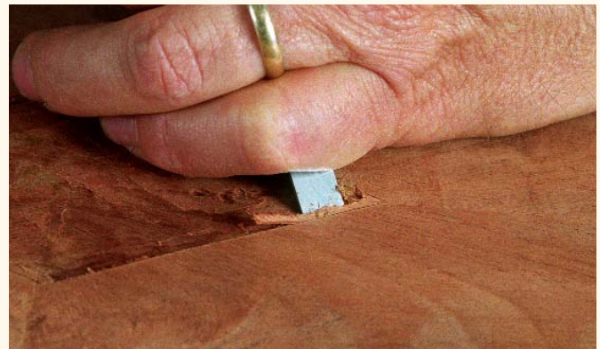
4 Clean up the cut with a chisel. Cut from the routed area into the waste using the knife cut as a stop cut.
