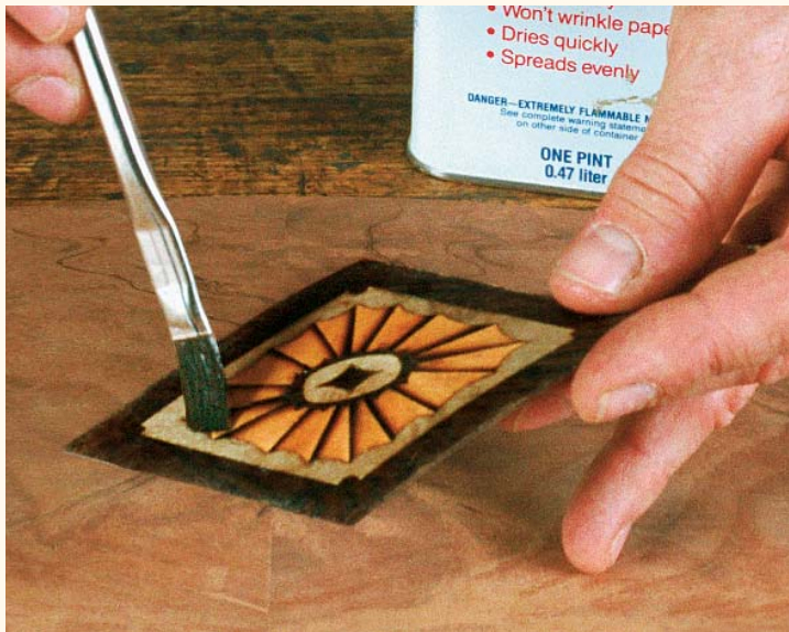
1 Cement the inlay to the tabletop. Apply a thin layer of rubber cement to the exposed side of the inlay. Then align the inlay carefully in the desired location and push it down.
