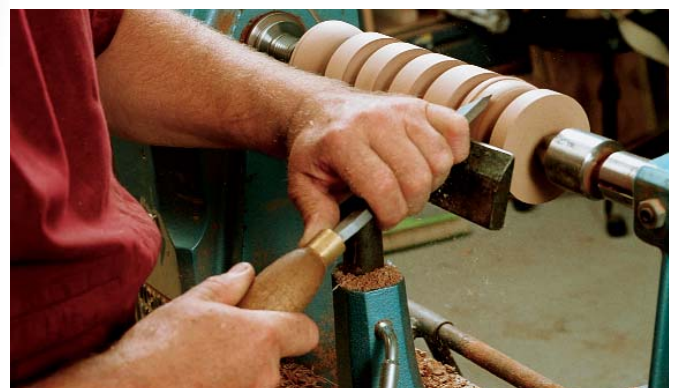
Overhand grip. The forward hand wraps around the top of the shank, and the tool rest supports the heel of the hand.
