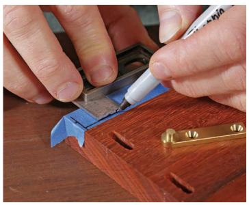
**Add a line for the setback.** This represents the back edge of the hinge and mortise. Use a small double square or combination square, and reference off the cabinet's front edge so that you can repeat the setback for every mortise in the cabinet.
