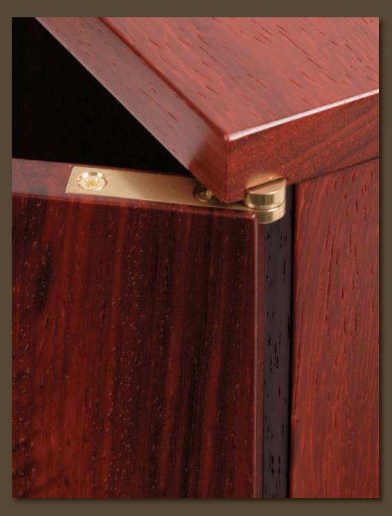
Inife hinges are perfect for the clean lines of the modern furniture I build. They are barely visible after installation and they're versatile, too. I've used them on small doors, large doors, flat doors, and even curved ones. Installing them can be difficult, because you must fit the door to its opening before you mortise for the hinge leaves, and even the smallest misplacement of the mortises can result in a door that doesn't swing properly and sits askew when closed.
