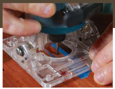
**Rout the waste.** Use a narrow bit—½ in. dia. works well—to clear out the mortise. Get as close to the tape as you can, moving slowly to improve control over the router.
