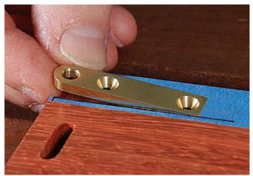
**Pare to the tape.** The tape's edge is like the line cut by a marking gauge. Put the back of the chisel against it and pare straight down (left). The hinge should slide in smoothly (above) but still fit snugly.
