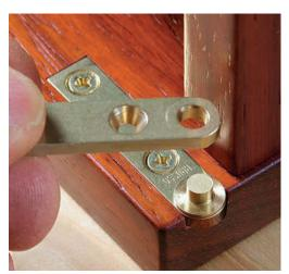
gap between the back of the door and the cabinet. Mark the mortise's location on the door's edge, and transfer this line to the door's bottom edge with a square. Follow the same process as for the cabinet mortises.
