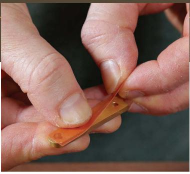
Tape the hinge to the cabinet. Press a piece of double-sided tape to the bottom of the hinge leaf (above). After exposing the tape's second sticky side, place the leaf on the cabinet, making sure that the line for the door's edge bisects the hinge barrel, and that the leaf is on the setback line (right).
