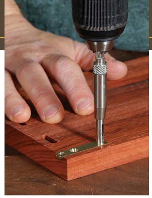
**Drill pilot** holes before assembling the case. A Vix bit automatically centers the hole, ensuring that the screw head seats properly in the hinge's countersunk hole.
