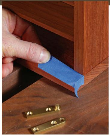
**Blue tape sets the stage.** Align the tape's back edge with the front edge of the cabinet side. It's OK for the tape to overhang the cabinet, but make sure that it's longer than the hinge leaf.
