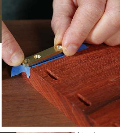
**Cut around** the leaf. With a marking knife, follow the hinge's perimeter, cutting through the blue tape.
