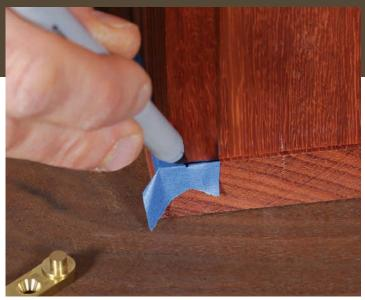
**Mark for the door's side.** After setting the door in place, trace along its edge. This line bisects the hinge pin.
