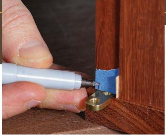
Mortise the door. With the hinge leaf in the mortise and blue tape on the door's edge, put the door in the cabinet and mark directly from the leaf's location. The process is the same as it was for the cabinet: Tape the leaf to the door, cut around it, remove the tape, rout the waste, and pare the walls.
