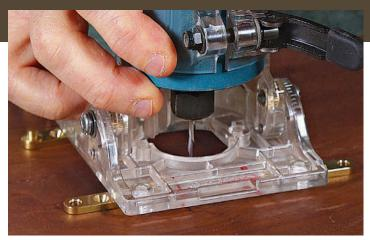
**Set the cutting depth.** Rest the trim router on four hinge leaves, and then lower the bit to the benchtop. Don't worry about compensating for the thickness of the blue tape.
