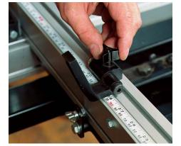
The flip-down stop on the Excalibur is located and locked along the fence's scale first. Then it's flipped down for use. The Exaktor's is almost identical.
