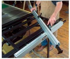
The Excalibur and Exaktor fences lock solidly. The clamping handles are easily accessible and easy to tighten. The angle scale on both fences is located on the extrudedaluminum outside rail, far from the pivot point, allowing fine graduations.
