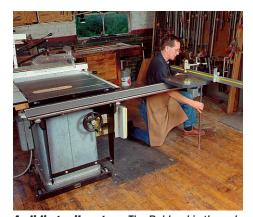
A sliding rail system. The Robland is the only model that delivers its full crosscut capacity with the fence mounted in front of the table (its only position). A stiff leg is added to support the heavy table and the work. The rails can also be slid to the rear.
