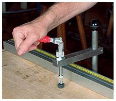
A workpiece hold-down is a necessity for accurate cutting. The Exaktor's hold-down clamp requires some practice. It's easy to apply too much pressure and thus flex the fence backward.
