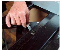
A table lock is handy. Both the Excalibur and Exaktor tables lock in place, which is helpful when loading large panels. A quick pull on the table unlocks it without having to reach underneath for a lock lever.
