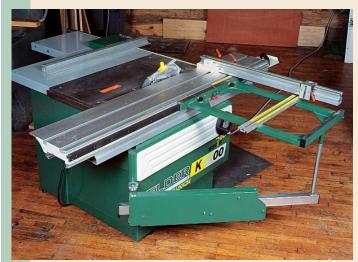
The ultimate in accuracy. After years of wrestling with sleds and other devices, the author bit the bullet and ordered the pricey but precise Felder sliding tablesaw. The sliding table is 78 in. long and runs right alongside the blade. And there are other European models available for less than the Felder.
