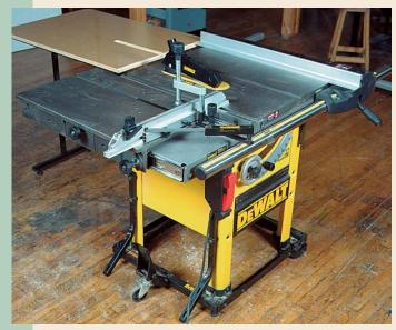
DeWalt's answer. With its recent tablesaw introduction (reviewed in FWW #140. p. 36), DeWalt responded to the need for accurate crosscutting. The 13/4-hp DW746 was designed for an accessory sliding table, placing it closer to the blade than aftermarket sliding tables can go. The DeWalt sliding table offers a 31-in. stroke, a cast-iron top, a welldesigned hold-down and a very solid feel.
