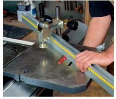
The Robland's angle scale gets you in the neighborhood. Miter angles can only be read roughly on the red scale inset into the table. The hold-down on the Robland is the stockiest of the three models. Large knobs fit the hand well, and the height is easy to adjust.
