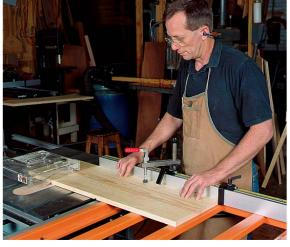
**Is your saw missing a sliding table?** One of these add-on units certainly will outdo your miter gauge and probably replace a few of your crosscut sleds. Difficult cuts such as large miters and multiple matching dadoes will be easier. However, the units examined here force you to choose between accuracy and the ability to support large stock.
