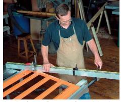
**Another innovative extension rod.** Another rod/extrusion combo can be mounted on the front or back of the table, allowing the Exaktor's fence to pivot past 90° and 45°.
