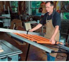
A quick-release bracket can replace the solid one on the Exaktor. This option is free if requested at the time of purchase. And one more of these brackets would make for a quick switch to a shaper.
